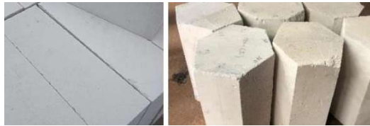
Figure 4. Stock AAC blocks from which test blocks were cut (left), and the cut prisms used in this study (right).
