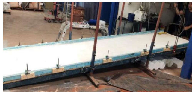
Figure 2. Photograph of the ramp used for the experimental testing (having its inclination adjusted).
