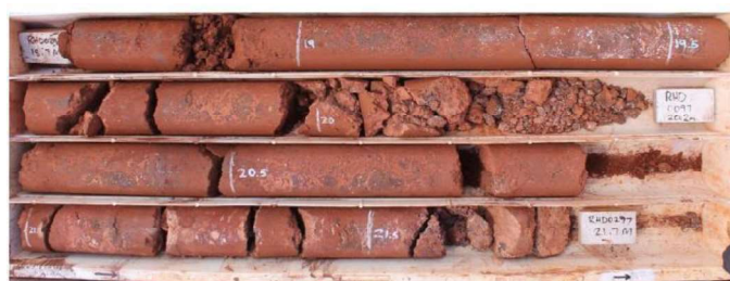
Figure 4. Hematitic conglomerate with cemented matrix.
