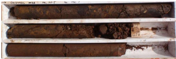
Figure 9. West Angela Shale – Brecciated/Sheared.
