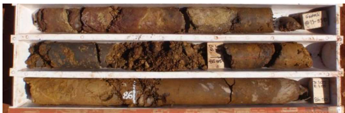
Figure 10. Extremely to highly weathered Paraburdoo Dolomite
