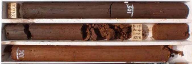
Figure 8. Extremely to highly weathered West Angela Shale (bedding mostly overprinted).
