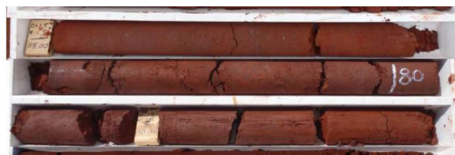
Figure 5 Hematitic conglomerate with poorly cemented matrix.
