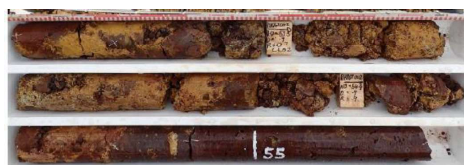
Figure 6. Duricrust or Canga/Hardcap with Clay Infill
