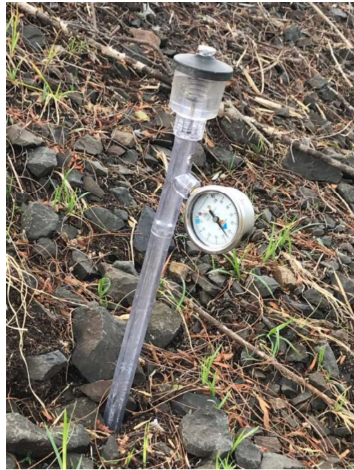
Figure 5. An installed soil tensiometer in action.
