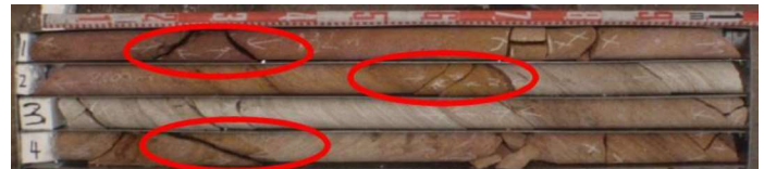
Figure 3: Typical sub-vertical joints encountered in an inclined borehole.
