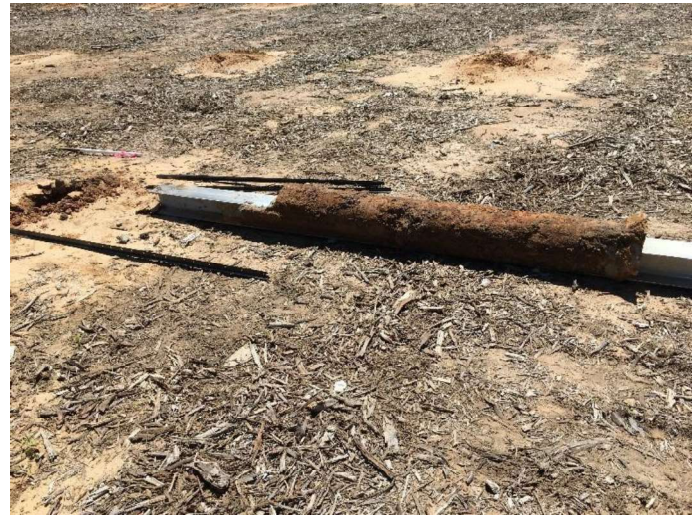
Figure 4. Extracted pile in stabilized sand.
