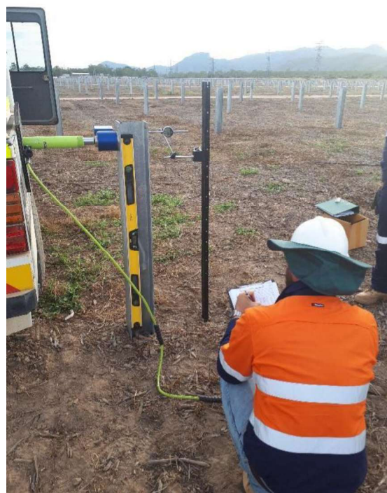
Figure 2. Typical lateral test setup showing jack, load cell and dial gauge. 1 dial gauge was used during proof tests as shown, 2 during design tests.
