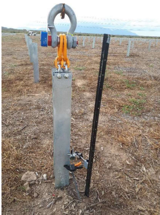
Figure 1. Typical axial test setup (lifting shackles, load cell and dial gauge shown)
