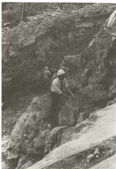
Fig. 2 - Slip surface on low-angle cleavage in meta-sediments.
