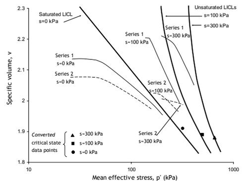
Figure 2: Isotropic compression tests, converted critical state data points (Sivakumar and Wheeler, 2000) and LICLs as adopted in the model
