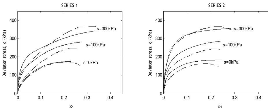
Figure 5: Experimental results (dashed lines) and model simulations (continuous lines) for constant suction triaxial compression tests in speswhite kaolin.
