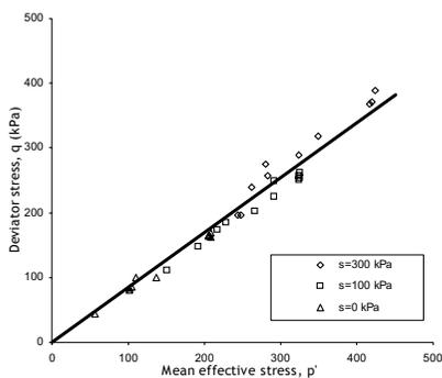
Figure 1: End points of a number of triaxial compression tests (Wheeler and Sivakumar, 2000)
