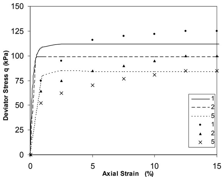
Figure 1: MCC prediction (continuous lines) and test data (symbols) of undrained stress-strain response of Anwara clay for OCR values of 1, 2 and 5
