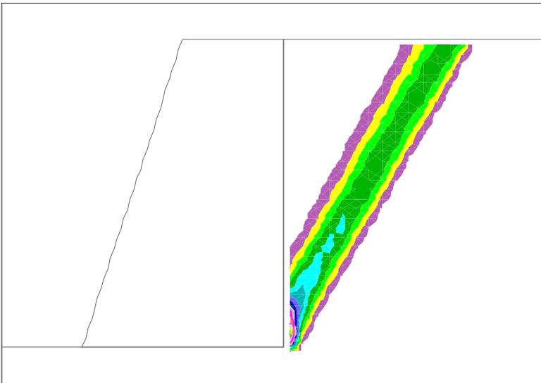
Figure 4: Contours of maximum shear strain rate for a smooth wall
