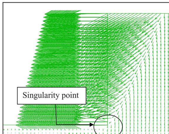
Figure 2: Displacement plot for active failure
