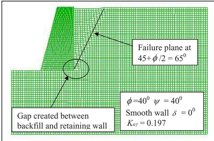
Figure 3: Exaggerated grid distortion of retaining wall model at active failure condition
