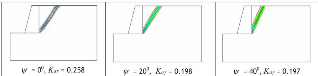
Figure 8: Variation in maximum shear strain rate and  $K_{ay}$  for various wall friction angles  $\delta$  and dilation angles  $\psi$  when angle of friction is  $40^\circ$  (smooth wall).
