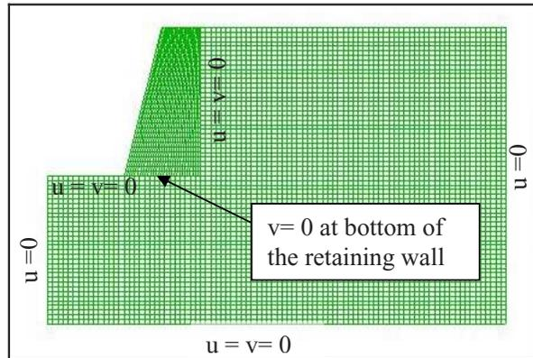
Figure 1: Boundary conditions of retaining wall model
