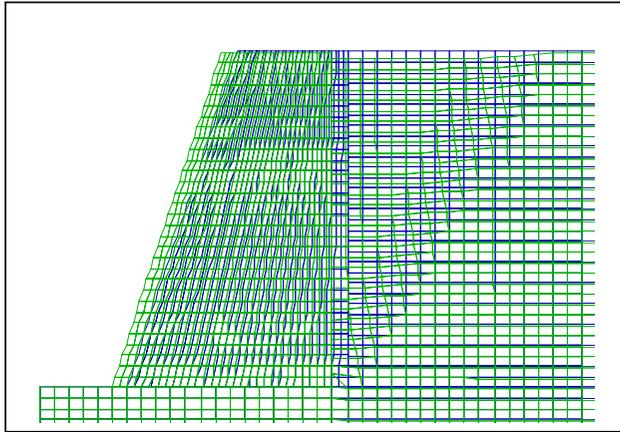
Figure 7: Sagging in the retaining wall backfill at active condition
