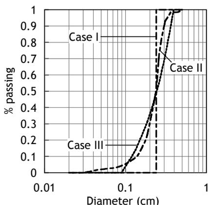
Figure 2. Particle size distribution
