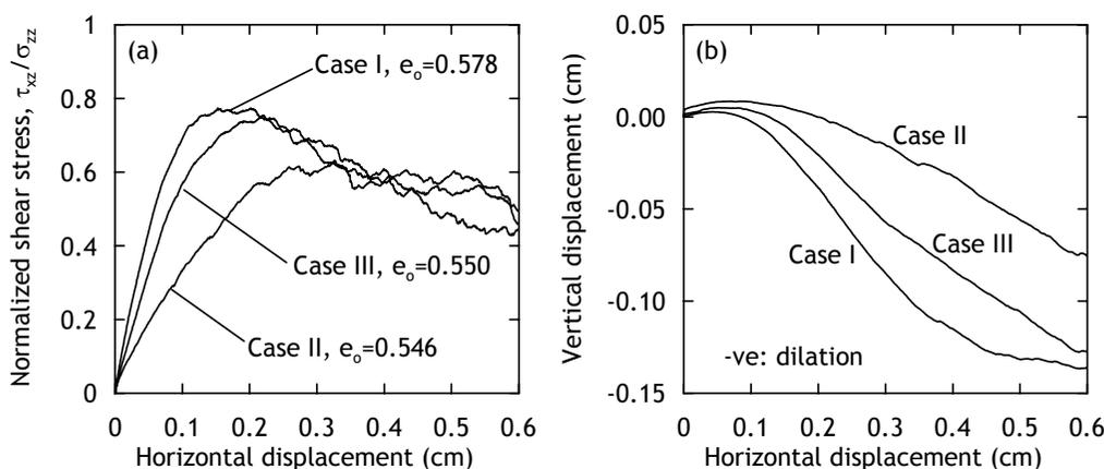
Figure 5. Responses of assemblages with different particle size distributions at  $\sigma_{zz} = 1$  GPa
