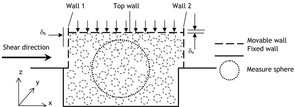
Figure 1. Schematic diagram of the numerical direct shear test
