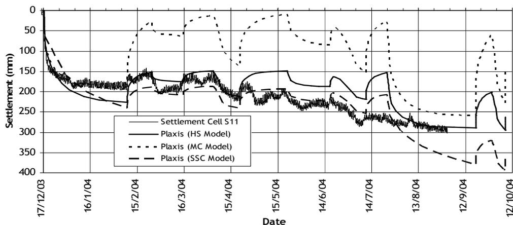
Figure 3 Vertical settlements beneath stockpile
