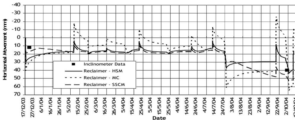
Figure 5 Horizontal movements at ground surface near reclaimer
