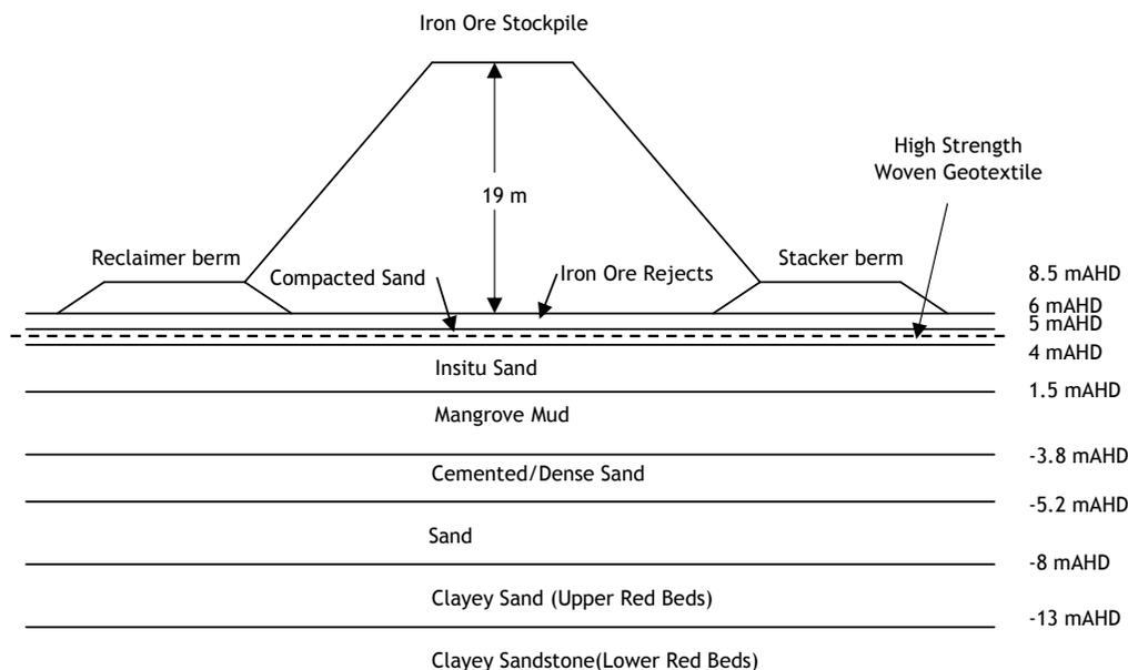
Figure 1 Schematic cross section through stockpile
