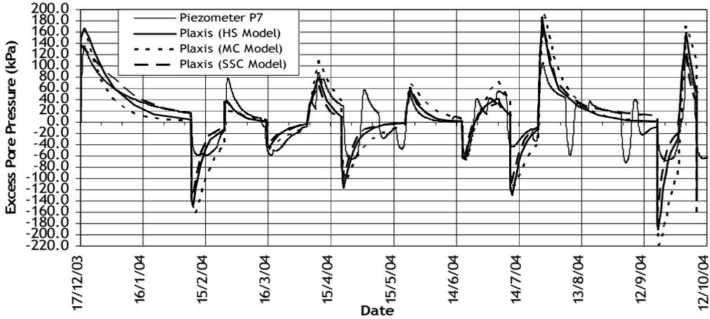
Figure 4 Excess pore pressures beneath stockpile
