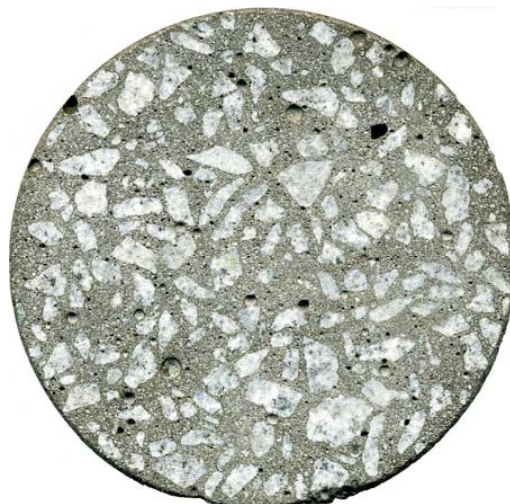
Figure 2: Curtin University of Technology 55MPa geopolymer concrete using 100% fly ash.
