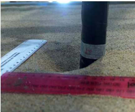
Figure 5: Soil displacement around the pile
