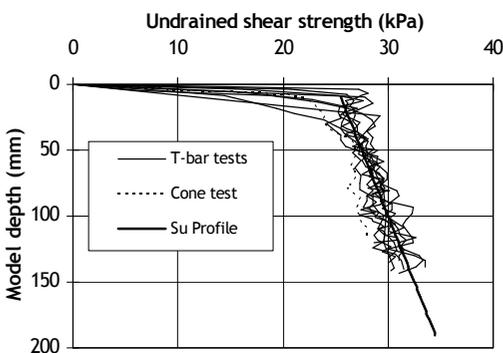
Figure 1: Undrained shear strength profile
