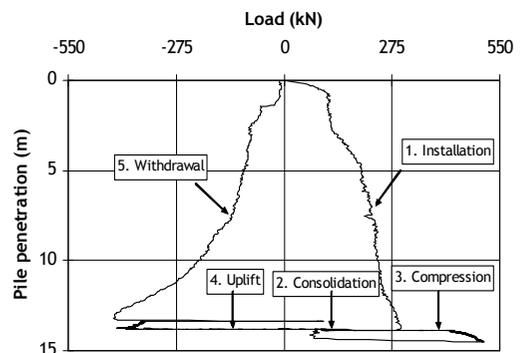
Figure 2: Stages in pile testing
