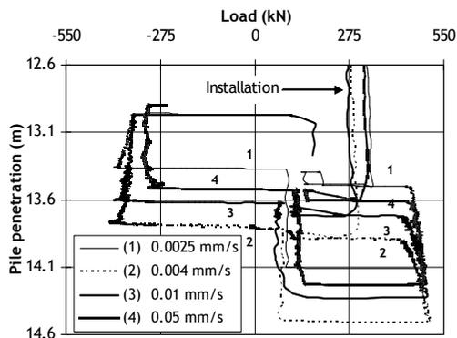
Figure 8: Effect of rate of loading
