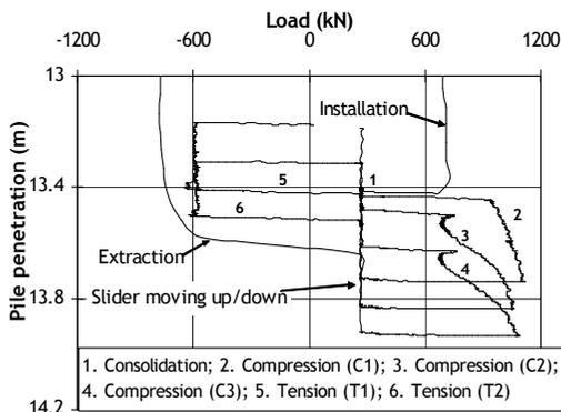
Figure 7: Effect of repeated loading
