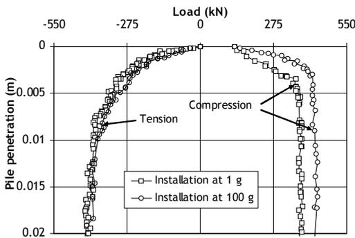
Figure 3: Effect of acceleration level
