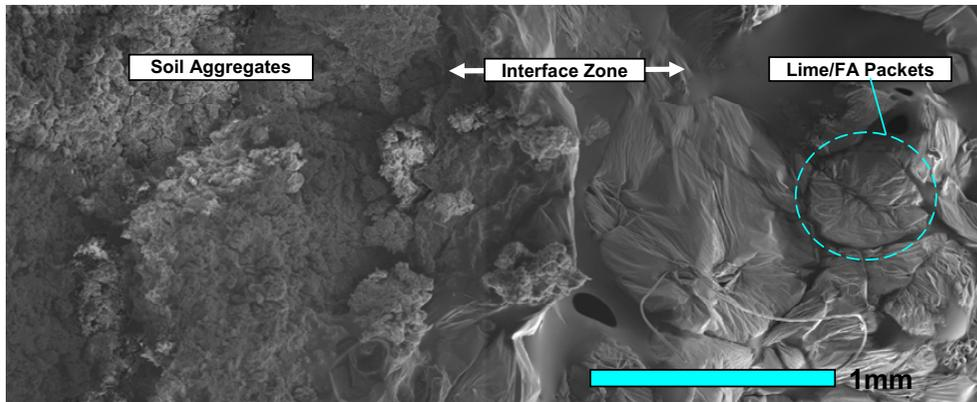
Figure 3: SEM image of soil and stabiliser physico-chemical interaction
