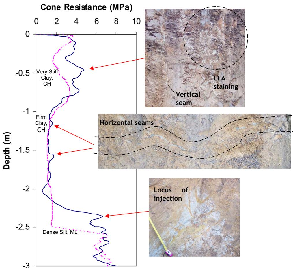
Figure 2: CPT trace of unstabilised soil profile (hatched line) and stabilised pad (solid line) with identified lime-flyash features
