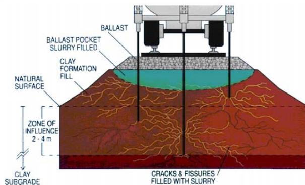
Figure 1: Pressure Injection of railtrack subgrades (Thiele and Adamson 2005)
