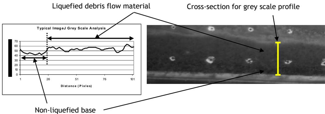
Figure 2: Grey scale intensity plot for non-saturation / saturation interface
