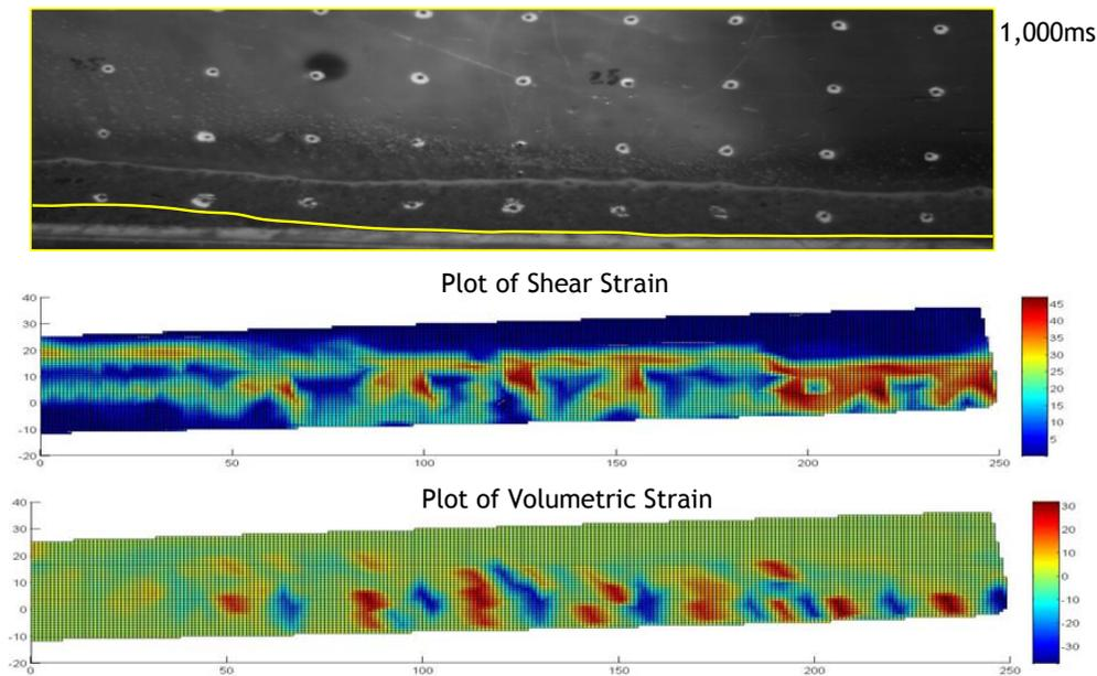
Figure 5: Saturation Interface and Strain Plots - Advancing bed erosion (1,000ms)
