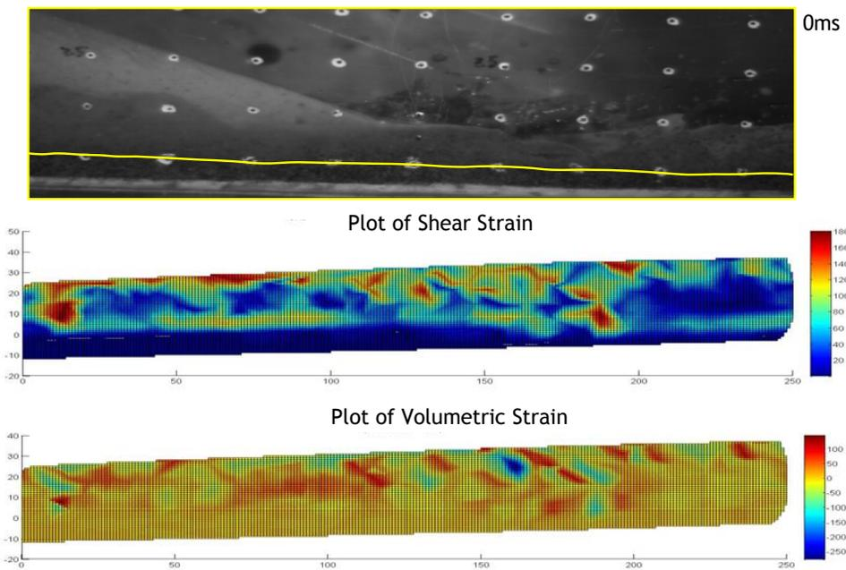
Figure 3: Saturation Interface and Strain Plots - Initial debris flow arrival (0ms)
