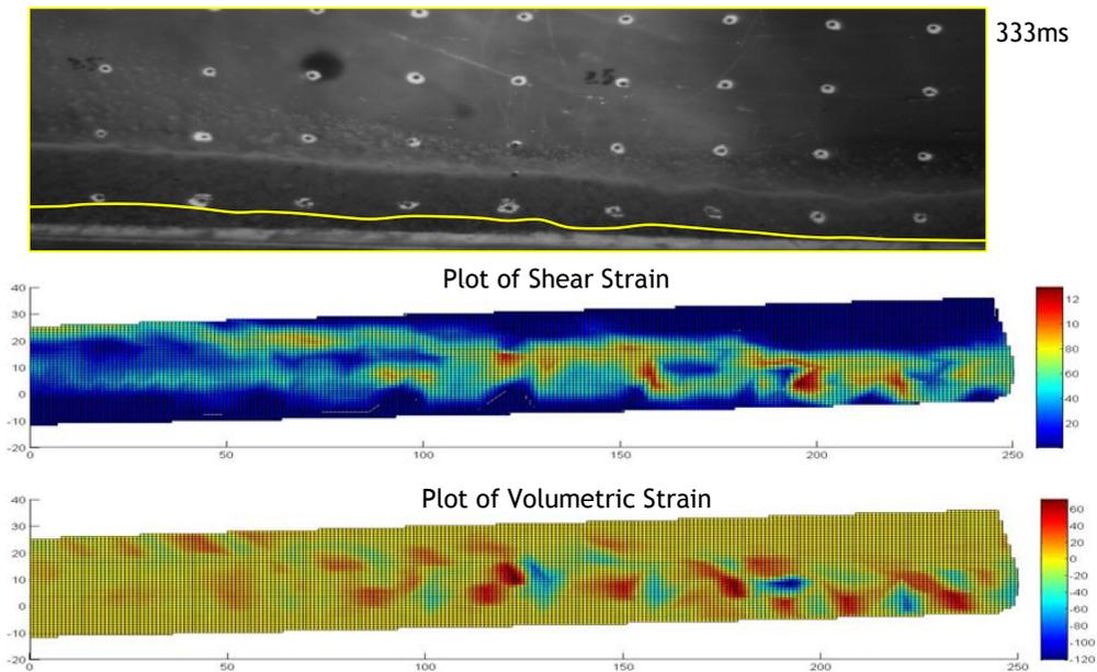
Figure 4: Saturation Interface and Strain Plots - Initial bed erosion (333ms)
