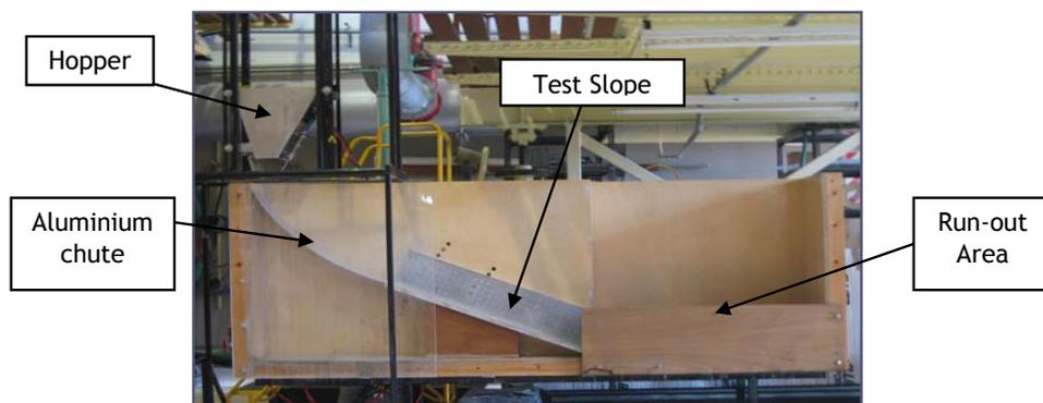
Figure 1: Testing Flume
