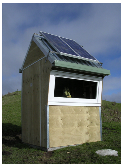
Figure 3: Monitoring hut and robotic total survey station. Power is derived from solar panels installed on the hut roof
