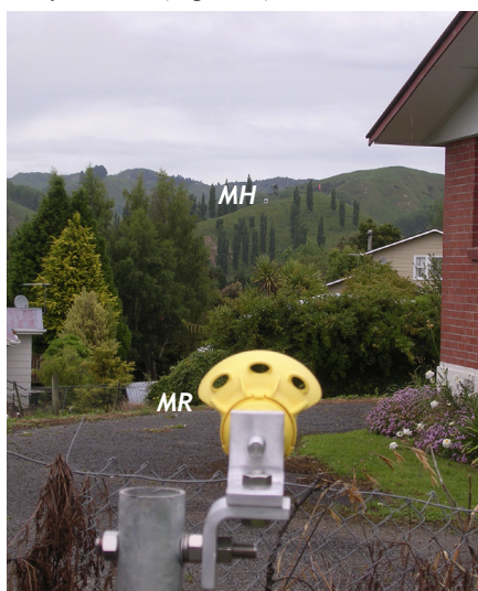
Figure 2: Monitoring reflector (MR facing towards the monitoring hut (MH), containing the robotic total survey station
