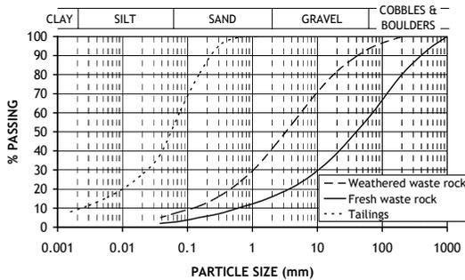
Figure 1: Particle size distribution curves
