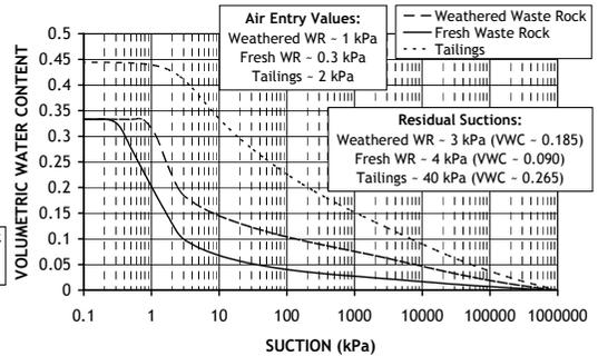
Figure 2: Soil water characteristic curves
