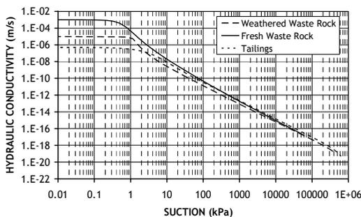
Figure 3: Hydraulic conductivity vs suction
