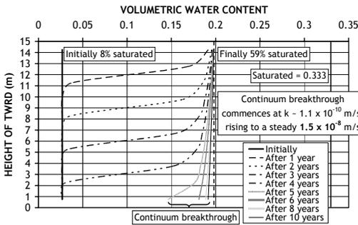
Figure 5: Wetting of weathered waste rock
