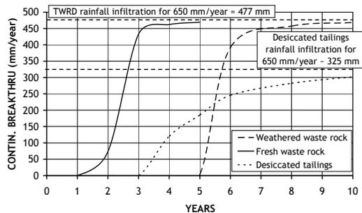
Figure 8: Time to continuum breakthrough
