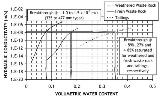
Figure 4: Hydraulic conductivity vs WVC
