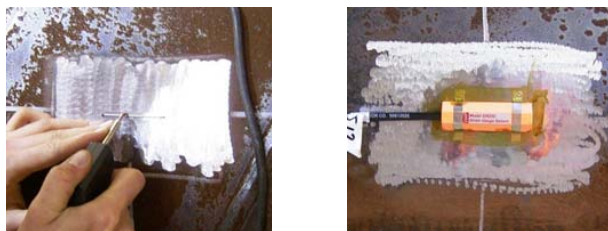
Figure 2 - Typical Strain Gauge Installation
