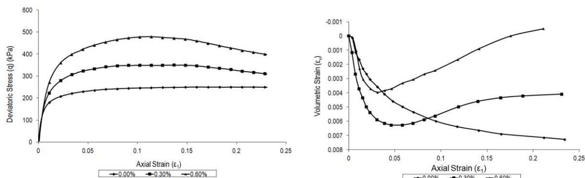
Figure 2: (A) Left: stress-strain behaviour of composite; (B) Right: volumetric behaviour of composite
