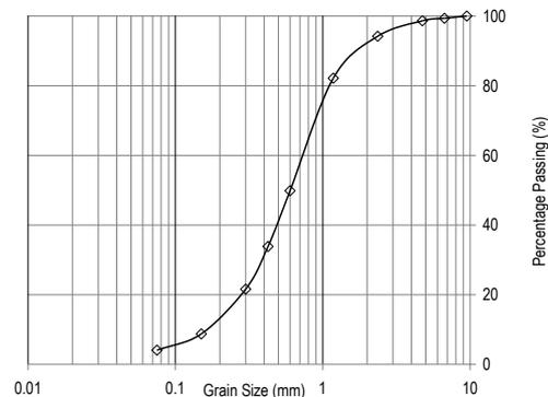
Figure 1: Particle size distribution for Prior Stream sand
