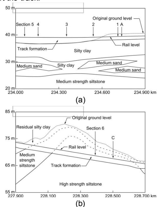
**Figure 2: Profiles of subsurface conditions of experimental sections**
