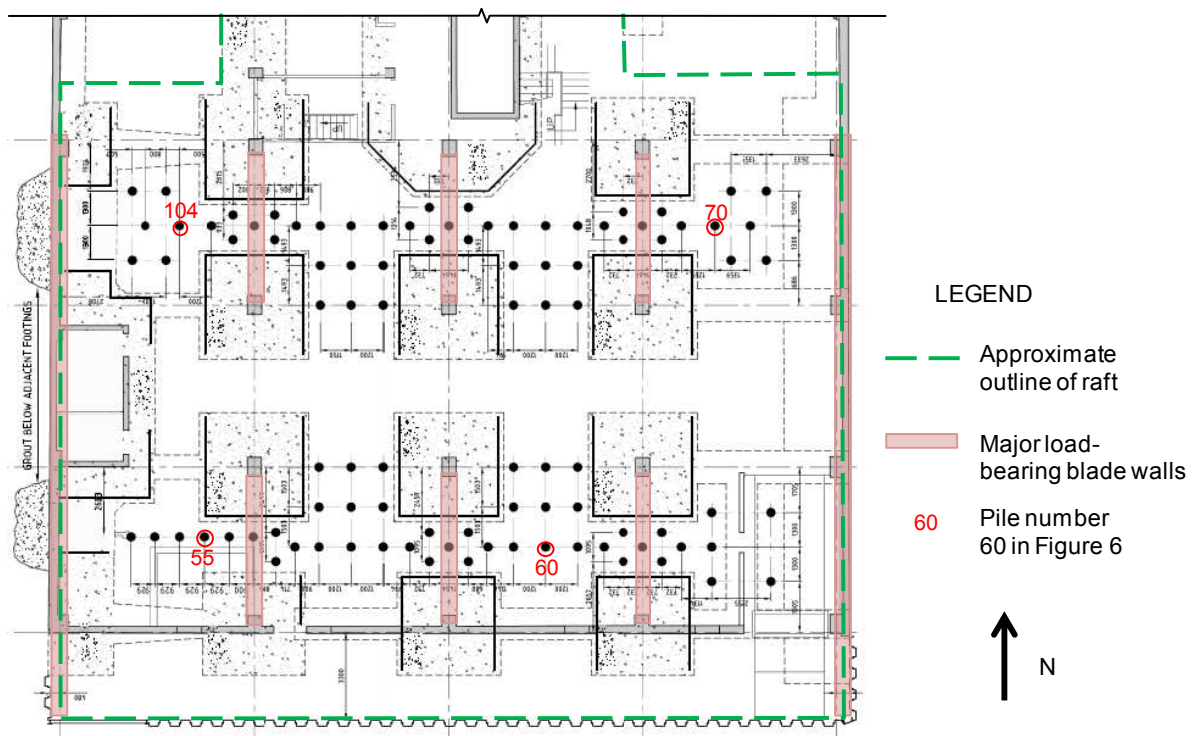
Figure 4. Micro-piles below new piled raft
