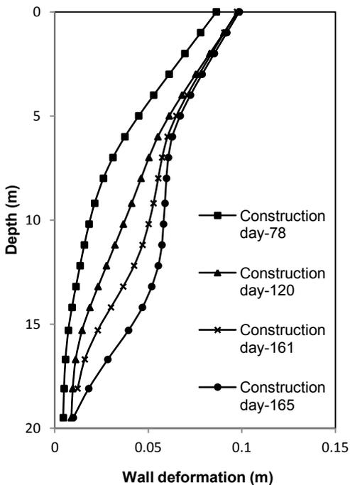
Figure 5. Wall deformation
