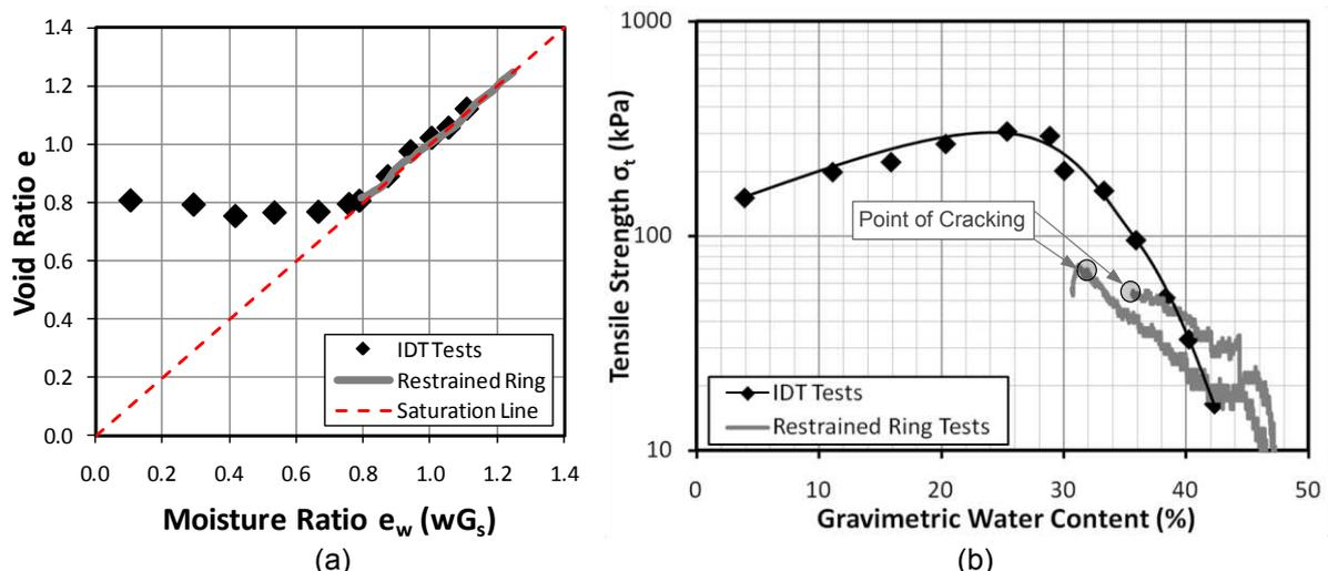
Figure 4. (a) Void Ratio vs. Moisture Ratio. (b) Tensile stress ( $\sigma_t$ ) vs gravimetric water content (%) and Comparisons between Restrained ring test and IDT tests.
