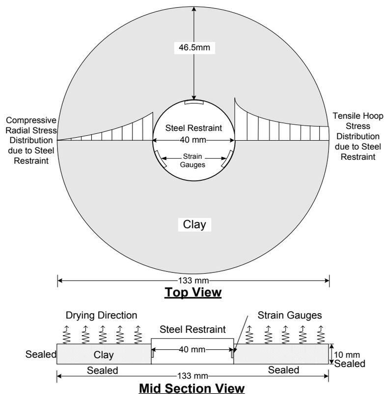
Figure 1. Restrained ring experiment dimensions and stress distribution
