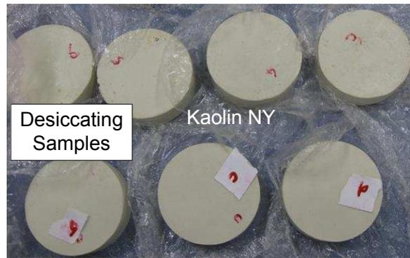
Figure 2. Cylindrical kaolin IDT samples during controlled desiccation
