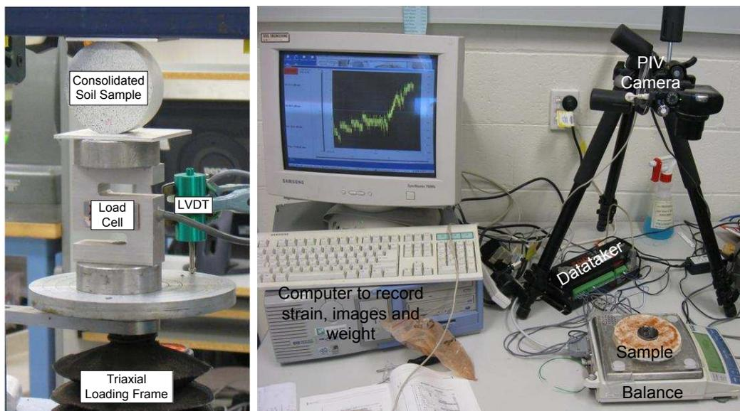
Figure 3. IDT loading arrangement for IDT cylindrical kaolin samples and restrained shrinkage tests (left) and testing arrangement for the restrained ring test (right)
