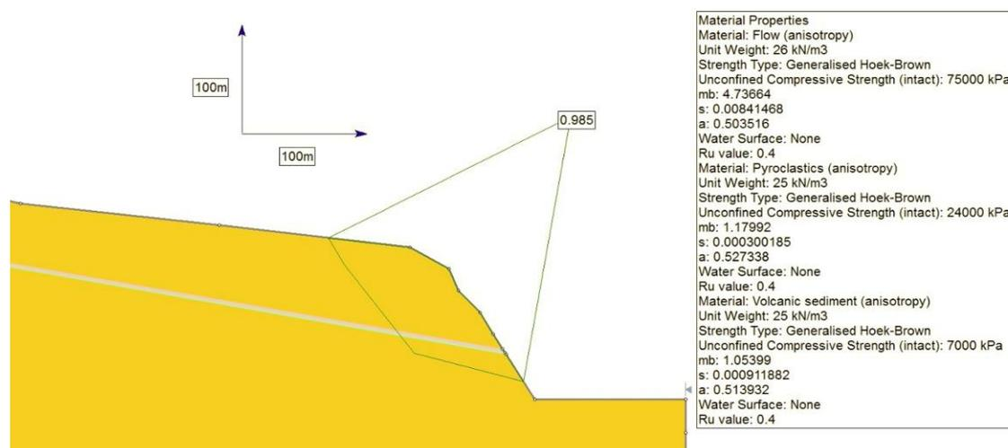
Figure 6 Output of minimum failure surface. The orange represents the Flow unit. The thin layers are Pyroclastics (beige) and Volcanic sediment (green).
