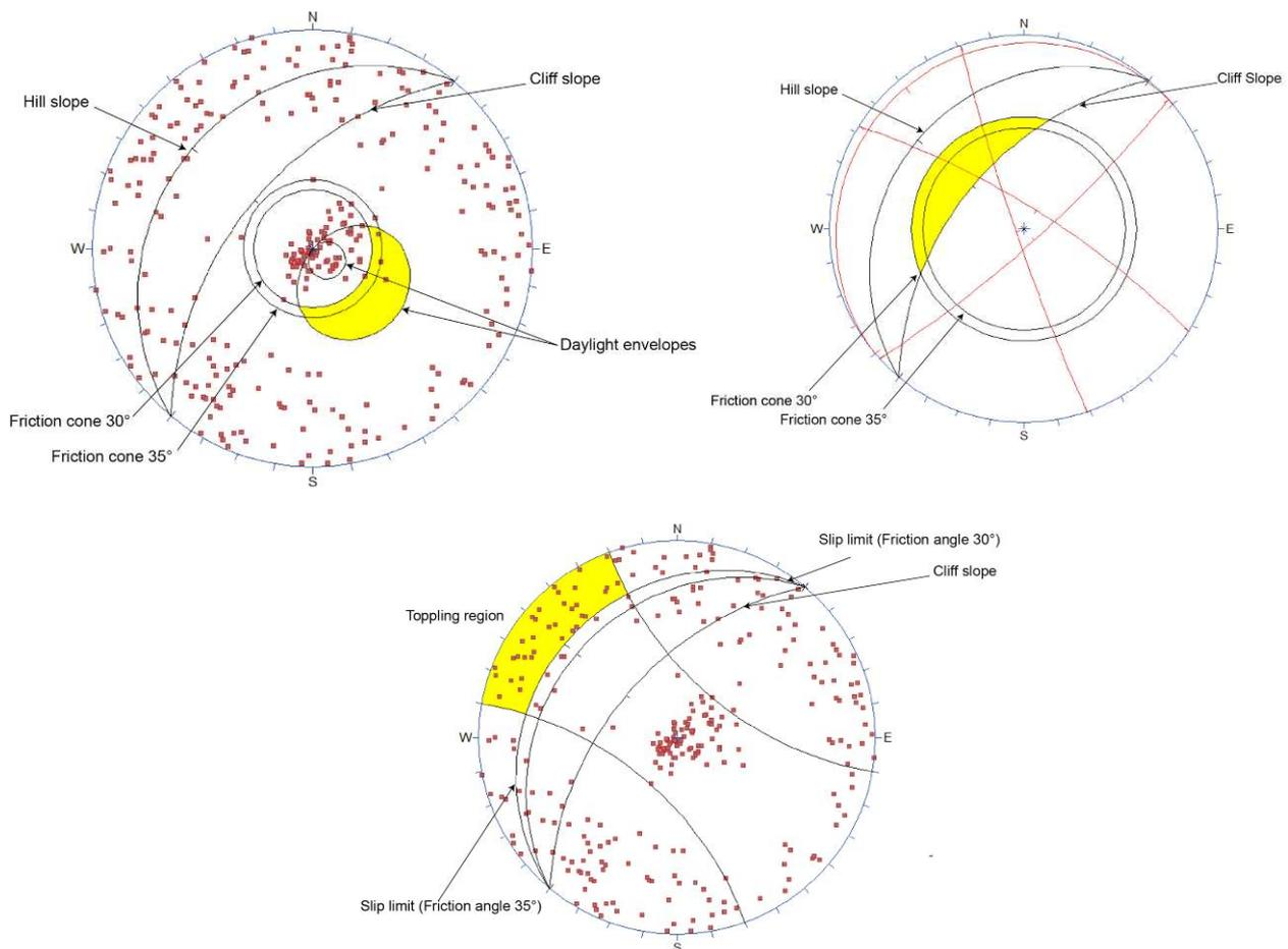
Figure 5 Kinematic analysis. A) Planar sliding. B) Wedge failure. C) Toppling.
