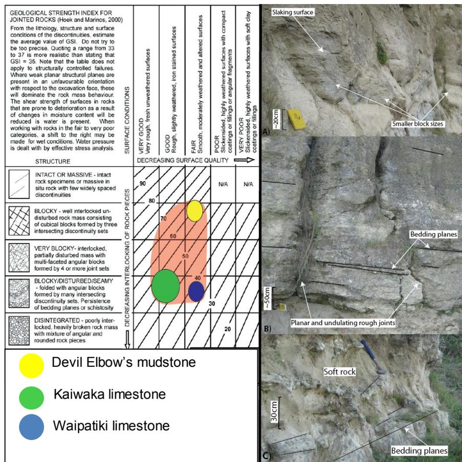
Figure 3: A GSI chart displaying rock mass quality for the different units, with the red circle displaying the overall range of values for the headscarp. Photo A) the Devil's Elbow mudstone; B) the Kaiwaka limestone; C) the Waipatiki limestone.
