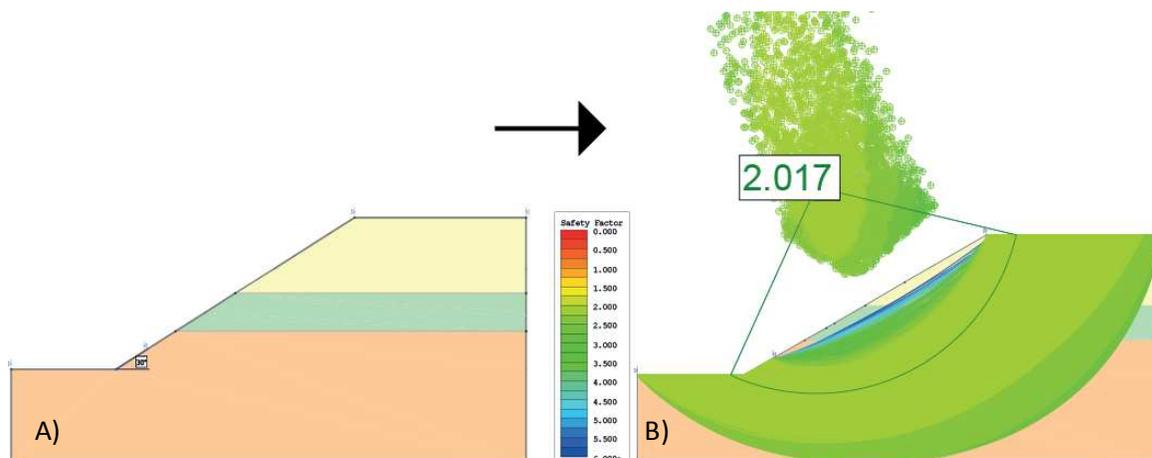
Figure 4: A) Model of the Tutira landslide headscarp with the three lithology layers displayed. B) The critical slip surface and FoS for the strong model without any pore water pressure or seismic loading.
