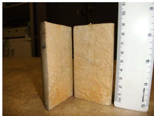
(a) fractured specimen
