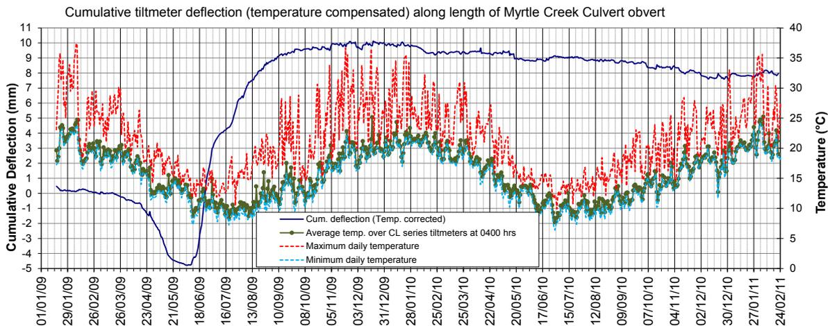
Figure 3: Seasonal temperature measured at MCC from tiltmeter derived data.
