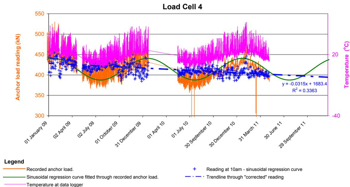
Figure 1: Response of Load Cell 4 - hourly readings versus time since January 2009.
