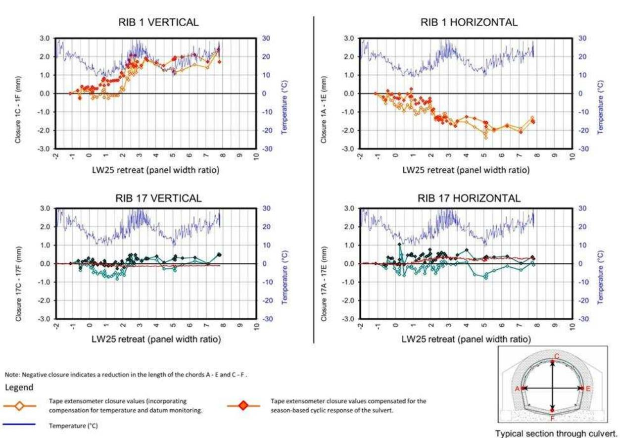
Figure 4: Response of two ribs within MCC to the retreat of LW25.
