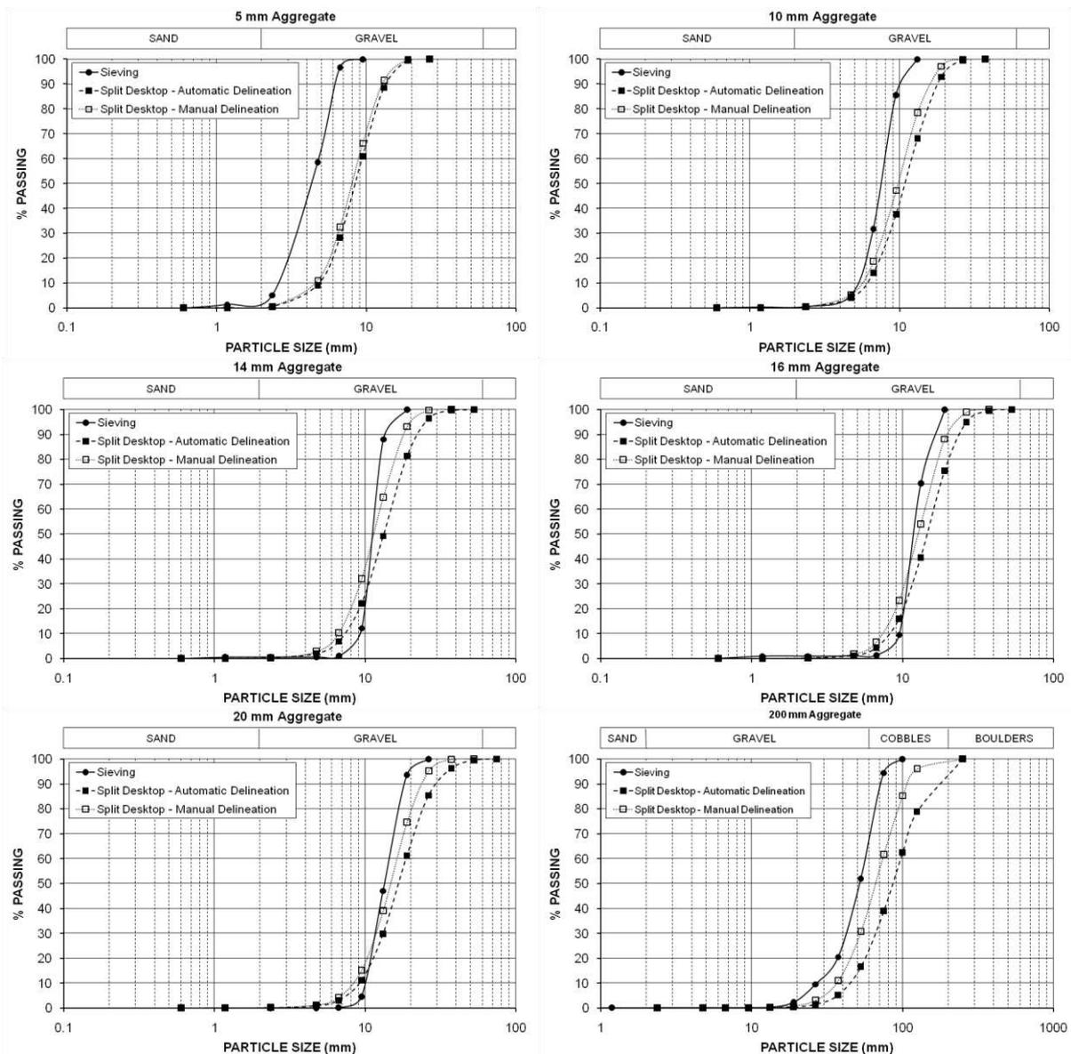
Figure 2. Split Desktop analysis results for 5 mm, 10 mm, 14 mm, 16 mm, 20 mm and 200 mm aggregate
