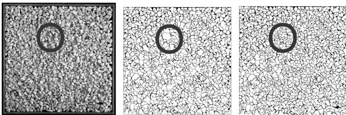
Figure 3. Comparison of the 14 mm aggregate: original image (left), automatic delineated image (centre) and manual delineated image (right) (Circle highlights an example of where automatic delineation has mistakenly grouped several particles together as one larger particle)
