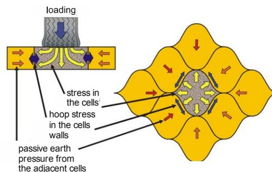
Figure 10. Schematic representation of the bearing mechanism of geocells (Emersleben 2010)
