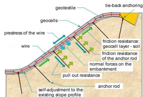
Figure 9. Erosion protection with geocells
