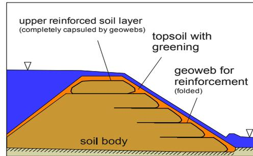
Figure 7. Sandwich construction by geosynthetics
