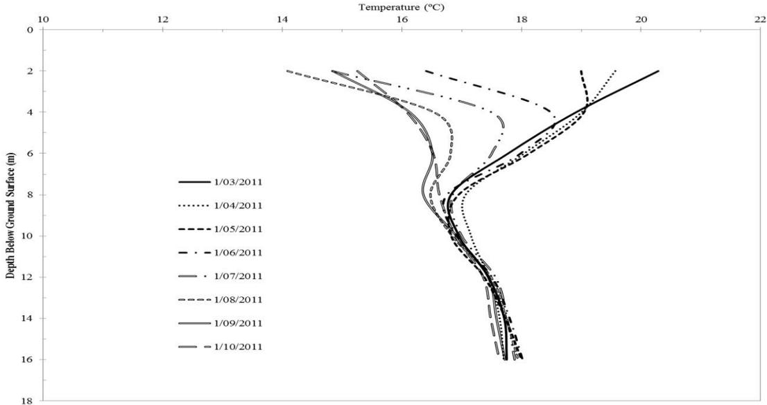
Figure 1. Typical temperature variation with depth recorded at Clayton
