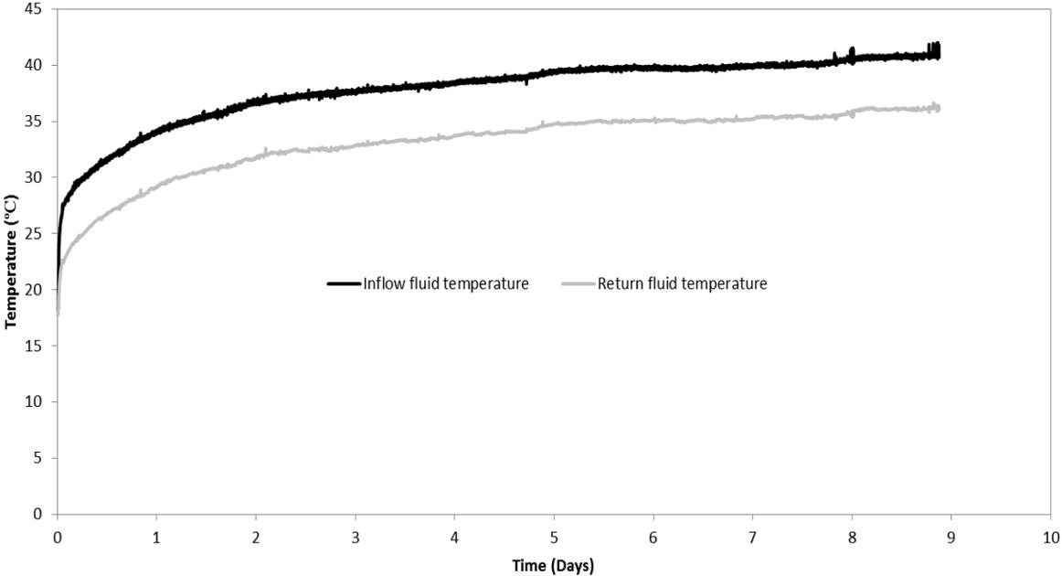
Figure 3. Thermal loading of the energy pile
