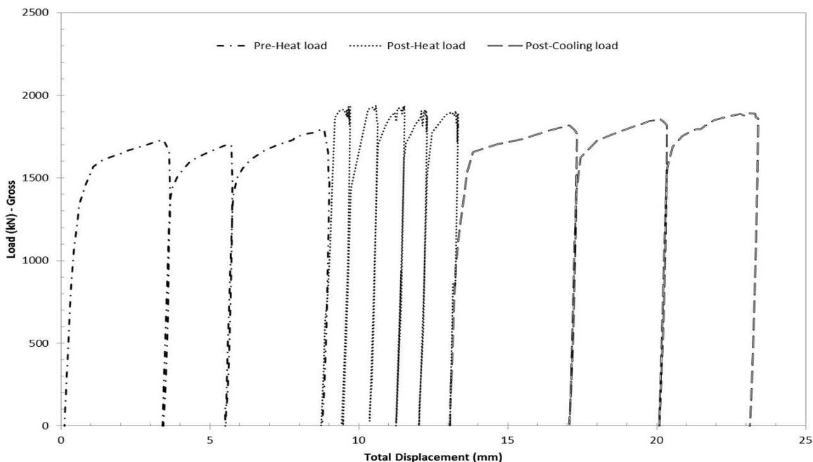
Figure 4. Ultimate pile shaft load before and after thermal loading
