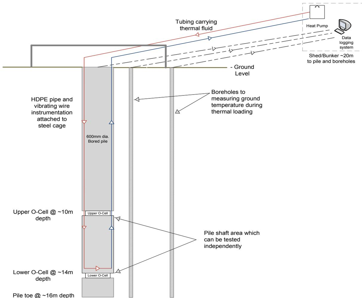
Figure 2. Field Energy Pile Testing Setup
