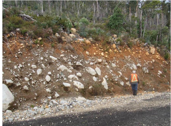
Plate 2: Ablation till exposed in a forestry road cut above the right abutment of the dam
