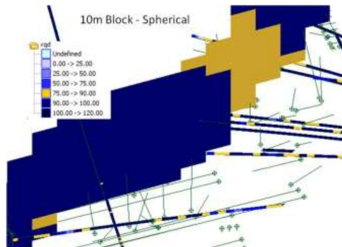
Figure 7. Comparison of interpolated RQD values in Model 2 and borehole RQD data
