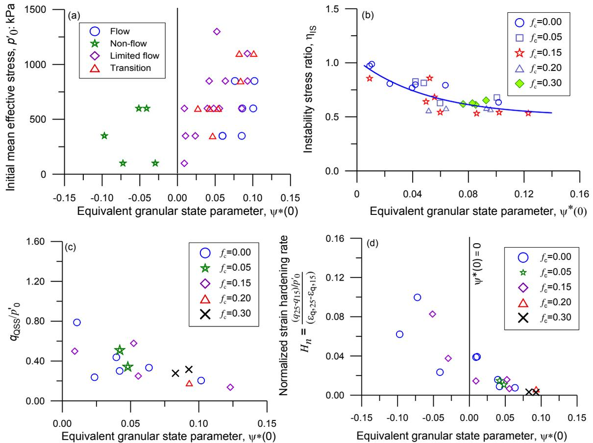
Figure 4: Relation between undrained behaviour and equivalent granular state parameter; (a) types of behaviour, (b) in  $\eta_{IN}-\psi^*(0)$  space, (c)  $q_{QSS}/p'_0-\psi^*(0)$  space, (d) in  $H_n-\psi^*(0)$  space
