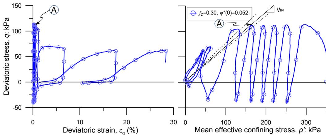
Figure 5: Prediction of cyclic instability behaviour for  $\psi^*>0$
