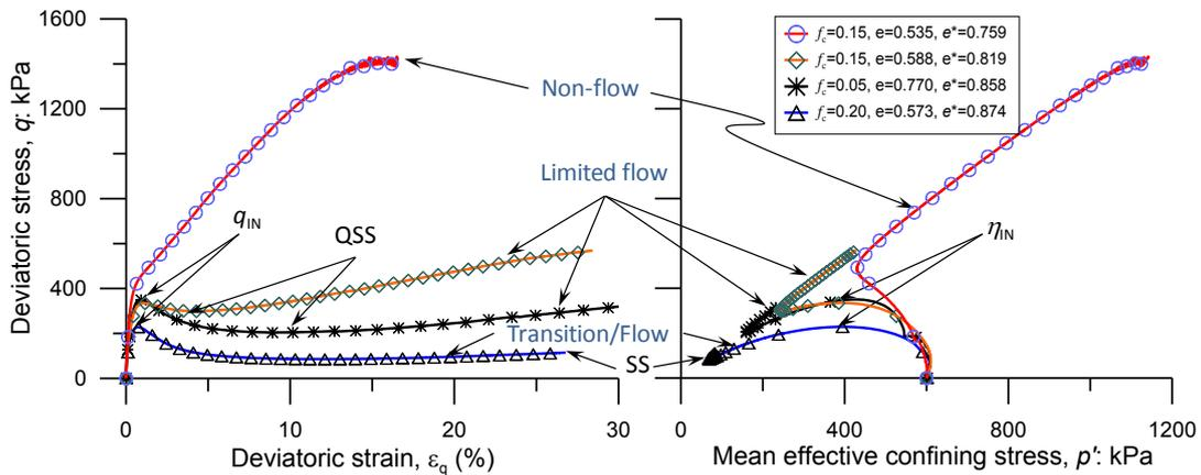
Figure 3: Type of undrained monotonic responses observed for sand with fines.
