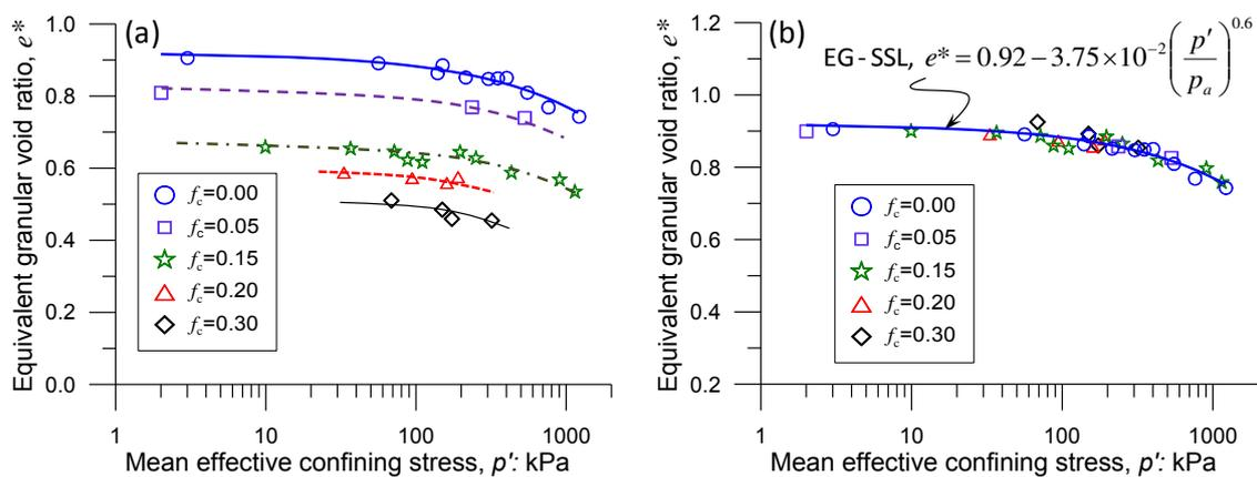
Figure 2: (a) SSLs for sand with fines; (b) EG-SSL for sand with fines
