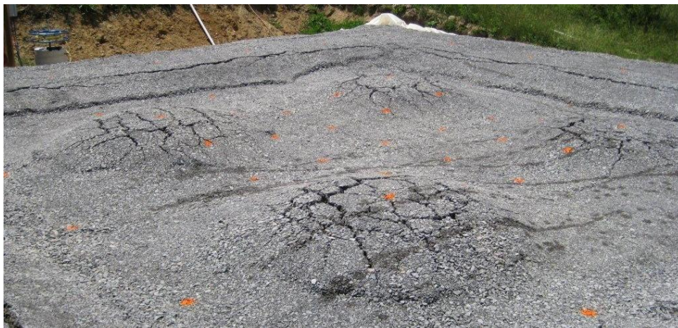
Figure 1. Mushroom Effect on the Surface of a Low Embankment Trial (Photo courtesy of Professor George Filz, Virginia Tech, USA)
