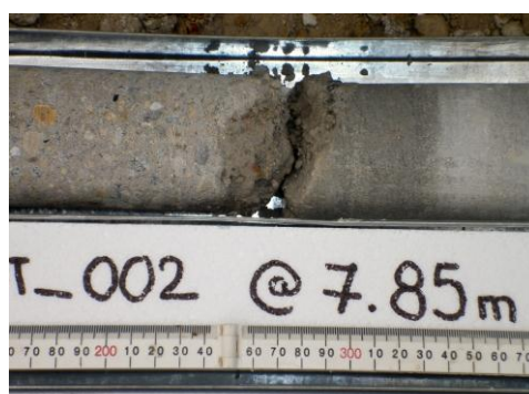
Figure 6. Flush contact between concrete and rock at base of test column T2
