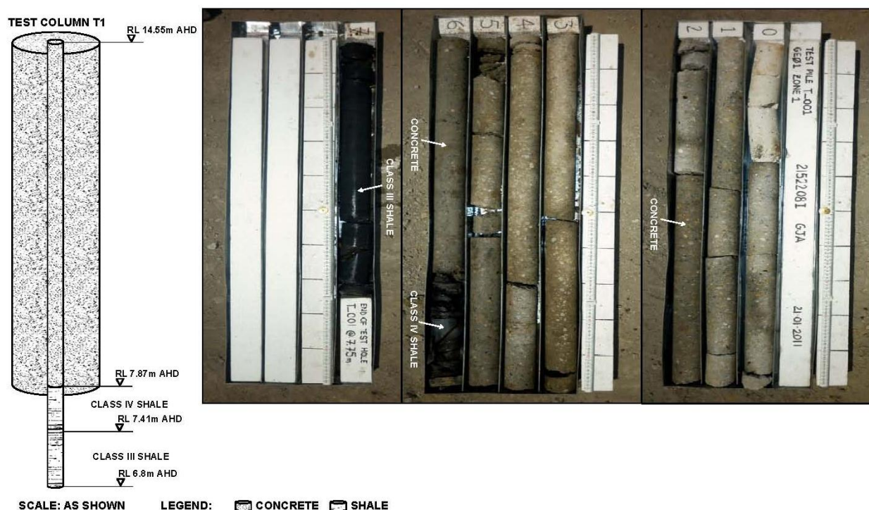
Figure 5. Coring test column T1
