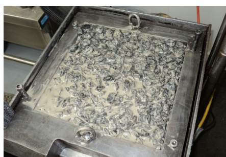
Fig. 6: Shear Box Test on Grouted Stone
