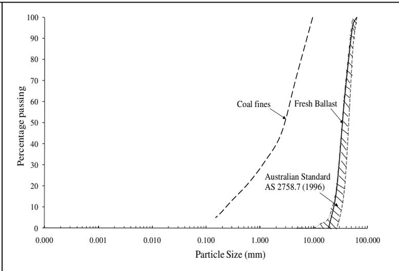
Figure 4. Grain size characteristics of fresh ballast and pulverised coal fines.
