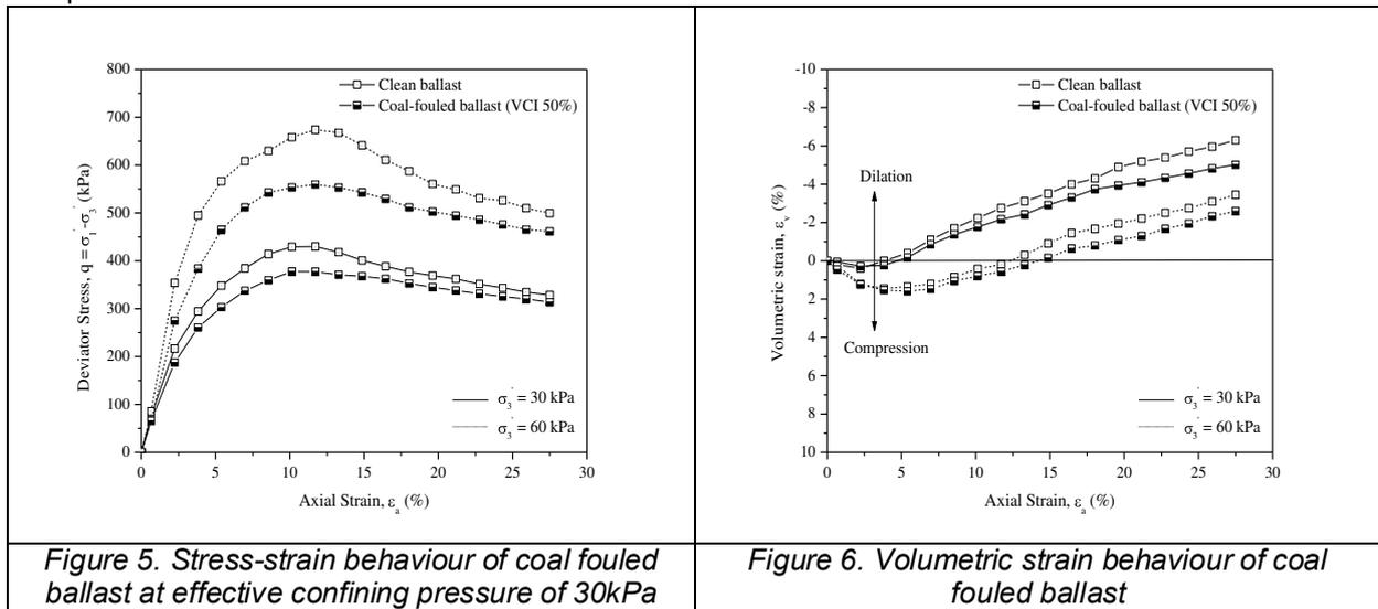
*Figure 6. Volumetric strain behaviour of coal fouled ballast*
