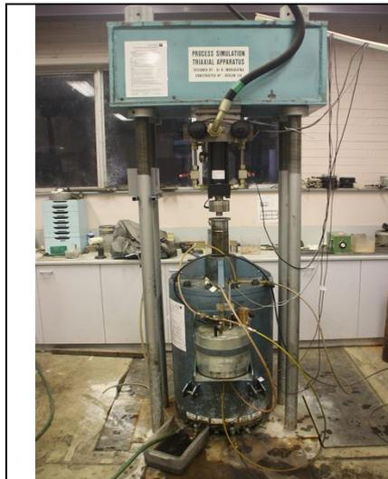
Figure 3. Large-scale cylindrical triaxial apparatus.
