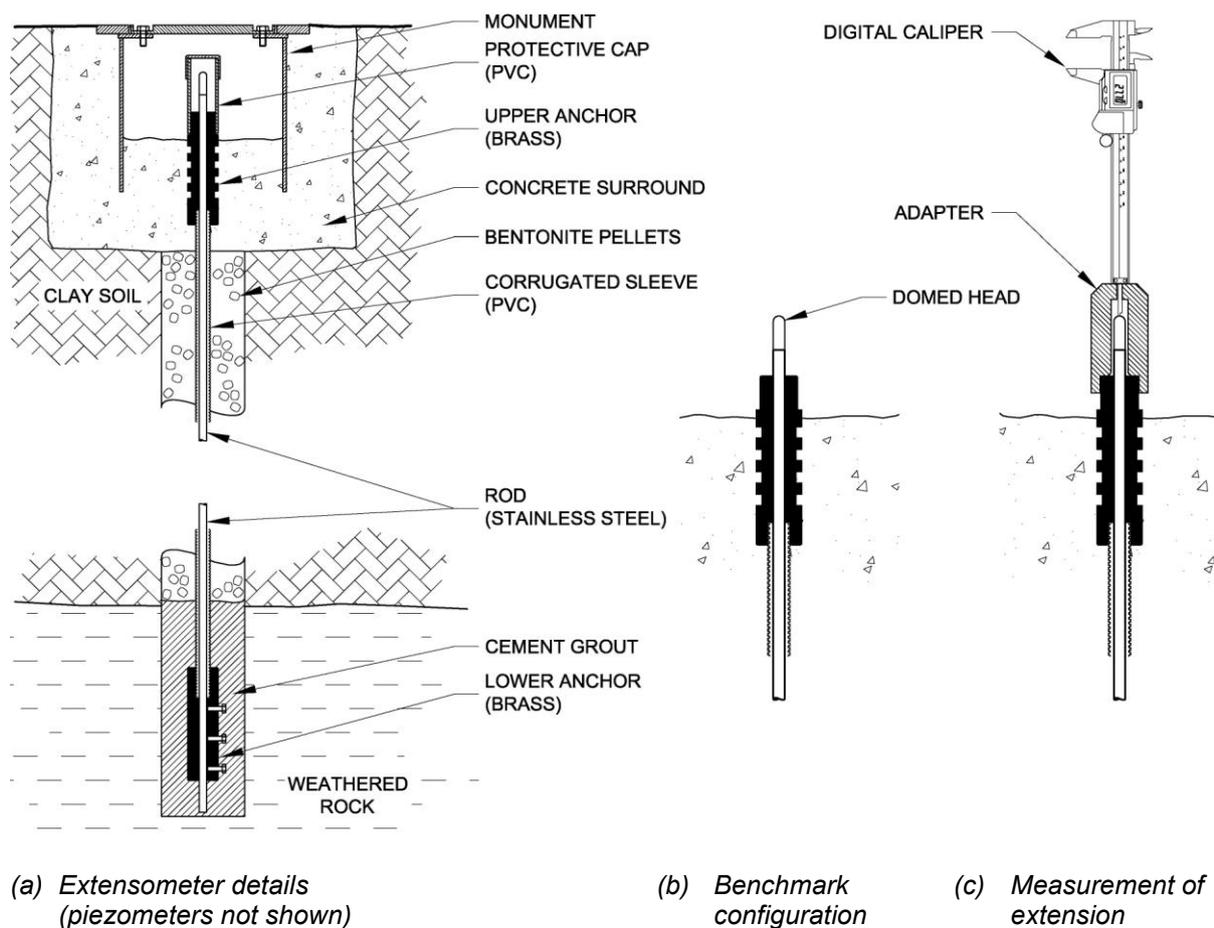
Figure 2. Extensometer details
