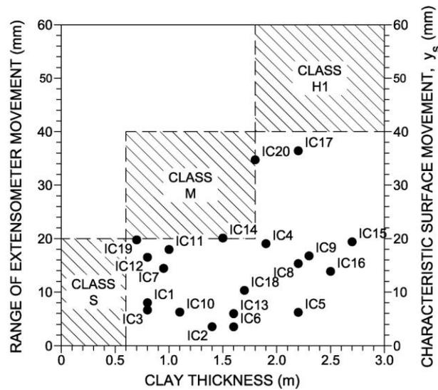
Figure 5. Clay thickness versus range of extensometer movement
