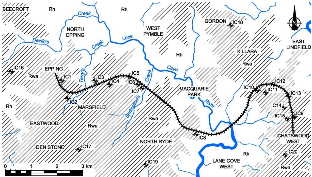
Figure 1. Plan of instrument cluster locations in relation to the tunnel alignment and geology
