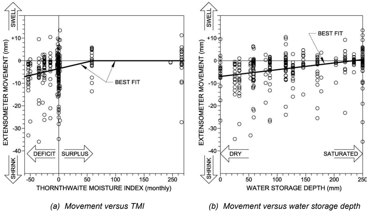
Figure 4. Ground surface movement versus TMI and water storage depth
