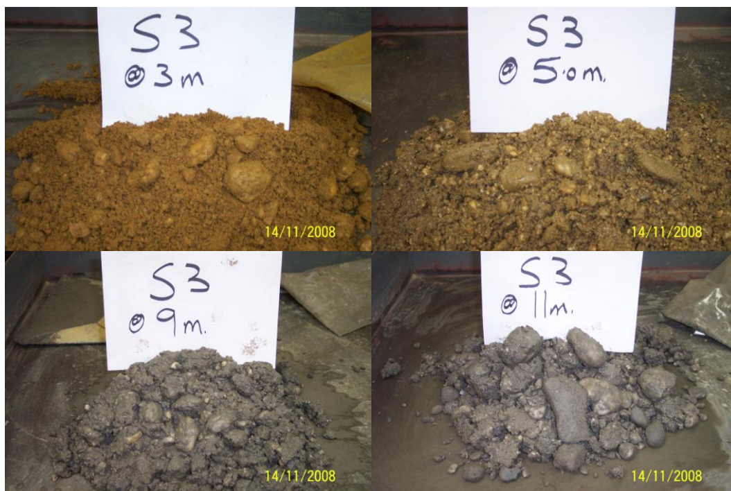
Figure 4. Soil samples showing alluvium particle size range collected using sonic drilling
