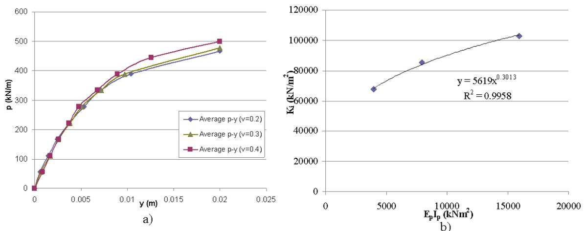
Figure 4 a) Average  $p$ - $y$  curves for different Poisson's ratios; b) Variation of  $K_i$  with different pile bending stiffness,  $E_p I_p$
