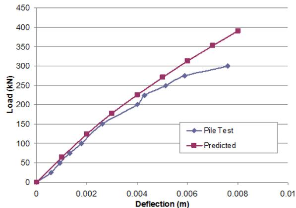
Figure 8 Comparison of pile head load-deflection of predicted pile test
