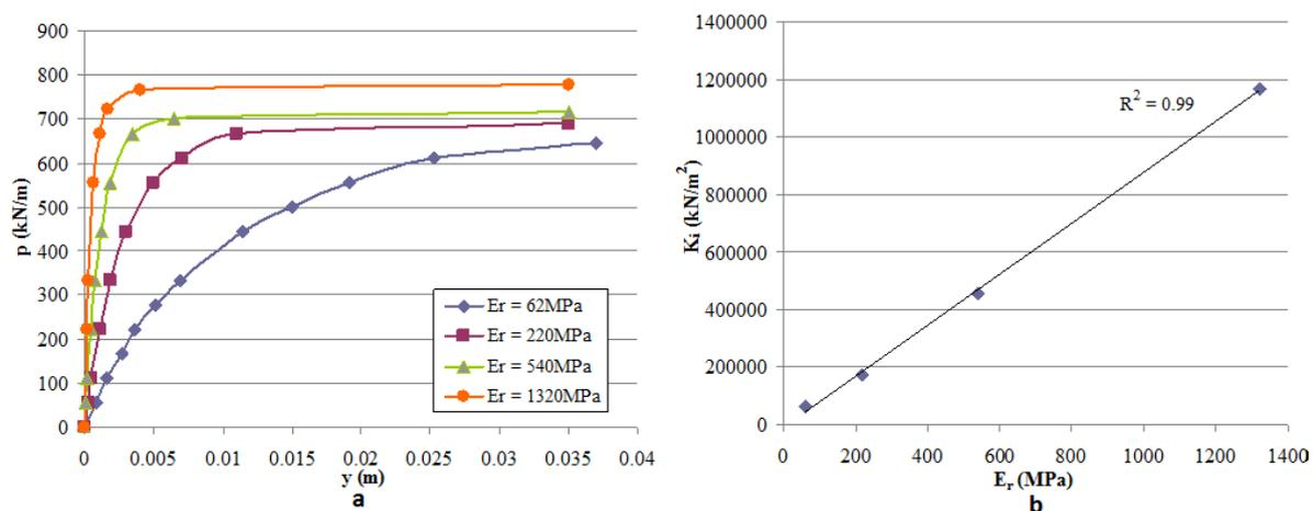
Figure 1 a)  $p$ - $y$  behaviour and b) Variation of  $K_i$  for different mudstone modulus
