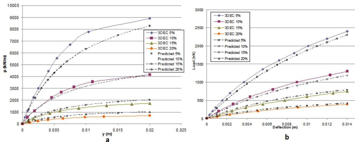
Figure 6 a)  $p$ - $y$  curves and b) Pile head load-deflection predictions using the proposed hyperbolic  $p$ - $y$  criterion
