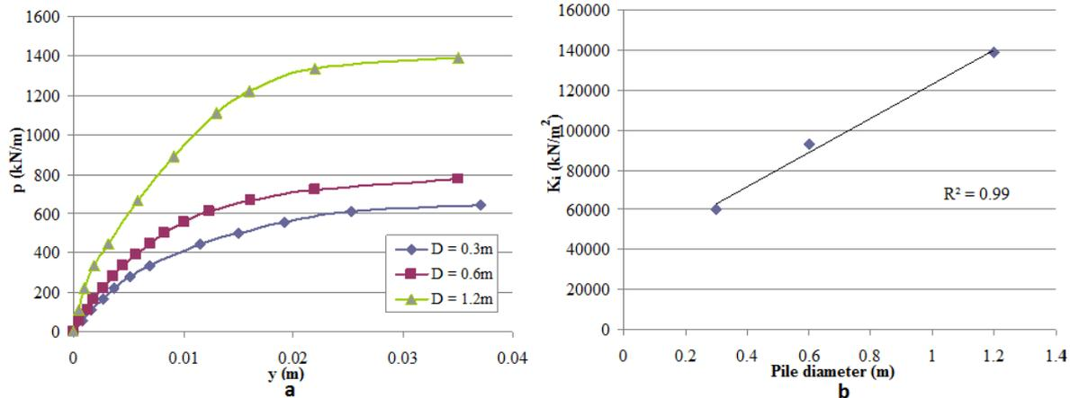
Figure 3 a)  $p$ - $y$  behaviour and b) Variation of  $K_i$  for different pile diameters
