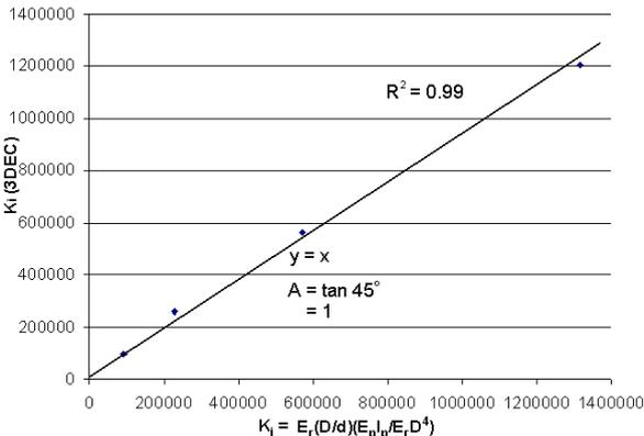
Figure 5 Comparison of 3DEC and predicted (Equation 4) initial subgrade reaction modulus
