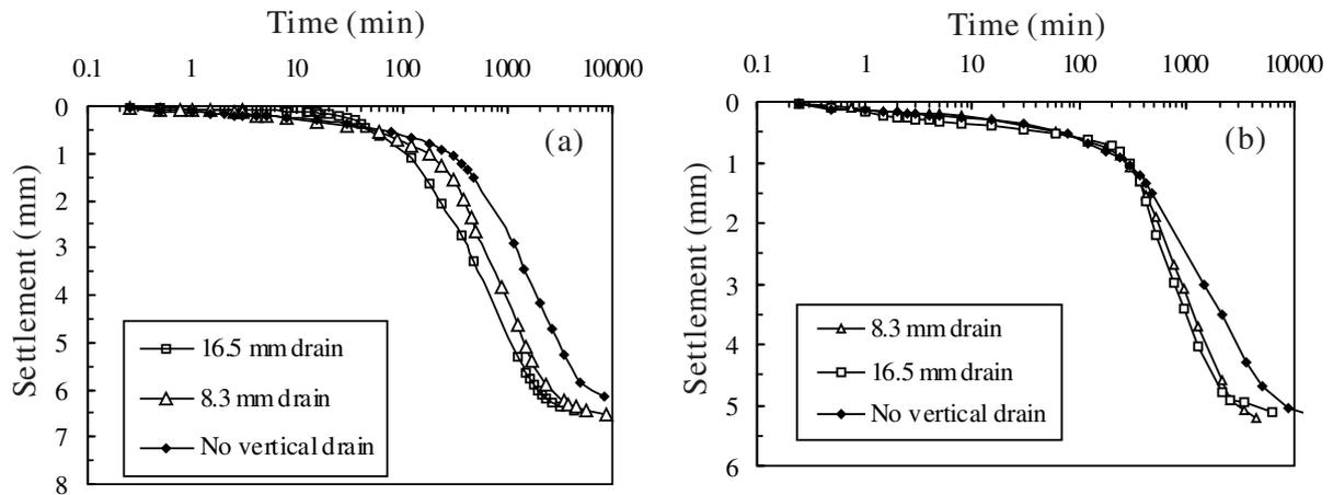
Figure 1. Results of Rowe Cell tests with and without vertical drains plotted as settlement against time at overburden pressures of 25 kPa (a), and 50 kPa (b).
