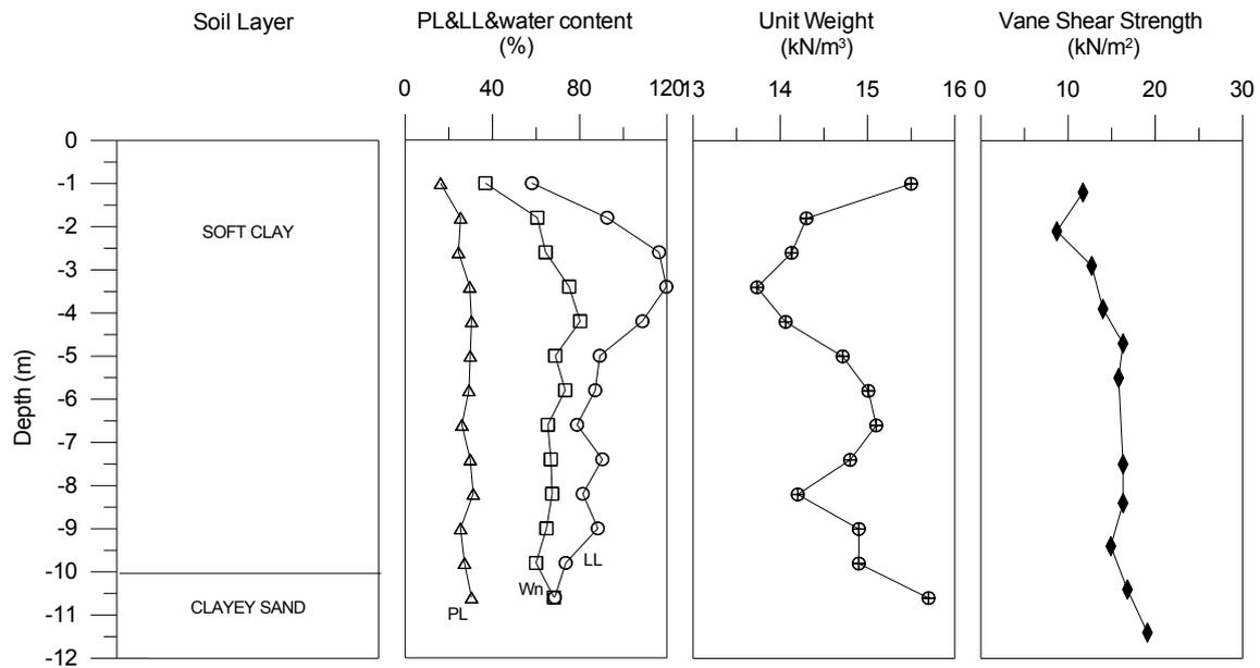
Figure 4. Geotechnical properties of soft clay at the trial embankment. PL-plastic limit; LL-liquid limit. (from Surarak 2005, Oh et al. 2007).
