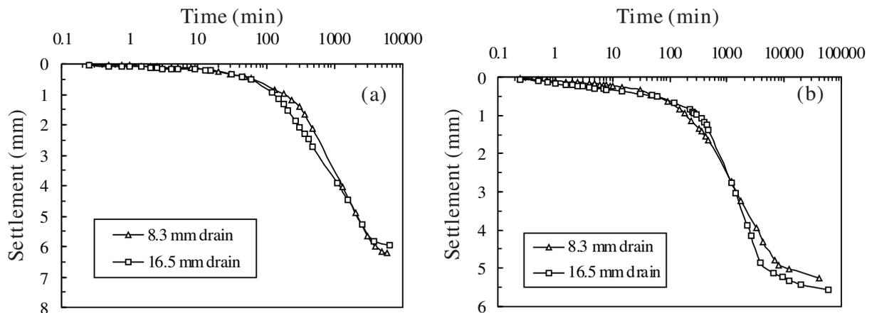
Figure 2. Results of Rowe Cell tests with and without vertical drains plotted as settlement against time at overburden pressures of 25 kPa (a), and 50 kPa (b) (with the smear effect).
