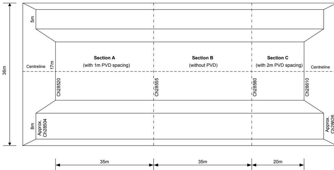
Figure 3. A schematic plan of trial embankment at the Sunshine Motorway (from Surarak 2005).
