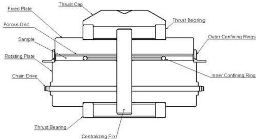
Figure 3: Section through main shear ring assembly (excluding drives, motors and housing)
