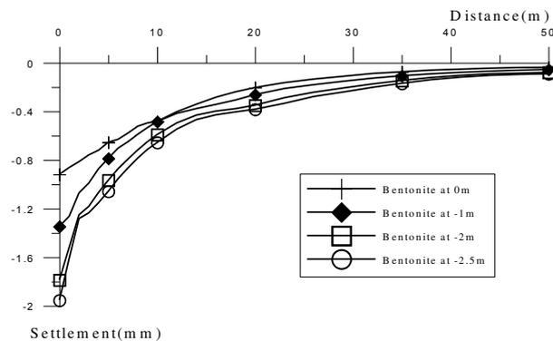
Figure 7. Surface settlement at the centre of trench on y-axis for different bentonite slurry height
