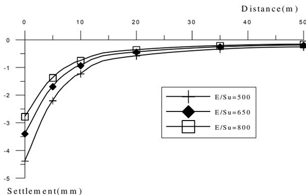
Figure 5. Surface settlement at the centre of panel on y-axis for various  $E/s_u$
