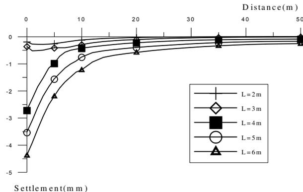
Figure 6. Surface settlement at the centre of trench on y-axis for different panel lengths
