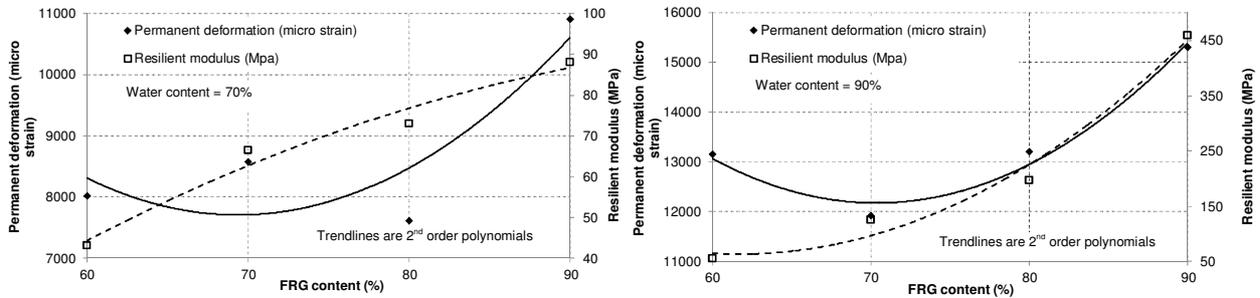
Figure 2. Change of permanent deformation and resilient modulus for FRG/Bio blends
