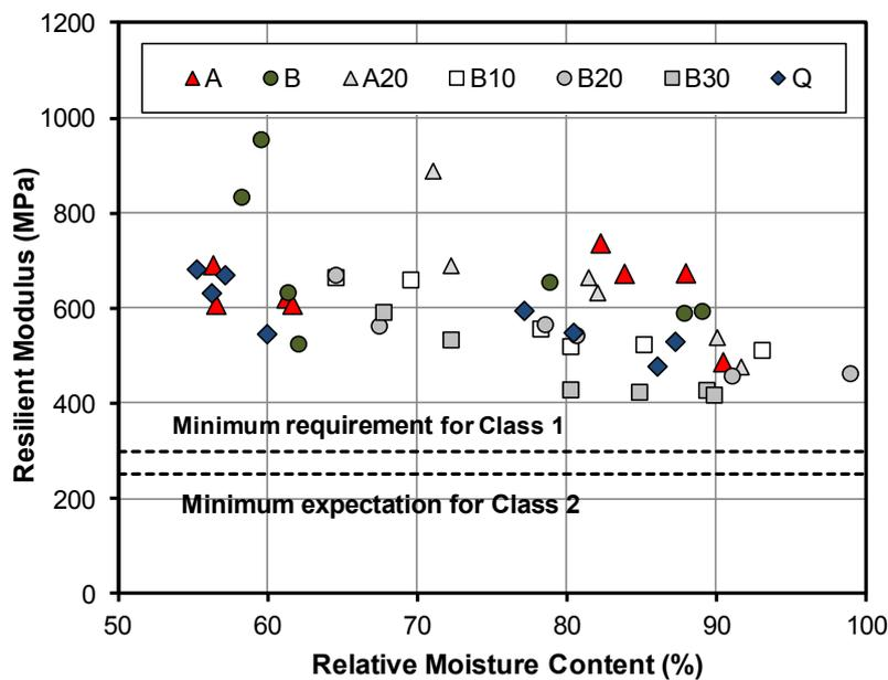
Figure 3. Resilient modulus as a function of initial moisture content
