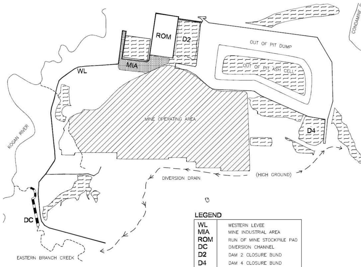
Figure 1. Schematic plan showing elements of Kogan Creek Mine flood exclusion system
