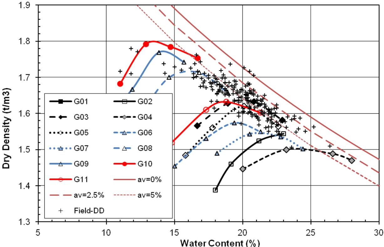
Figure 3. Comparison of field compaction with initial laboratory testing, air voids lines for  $G_s=2.64$
