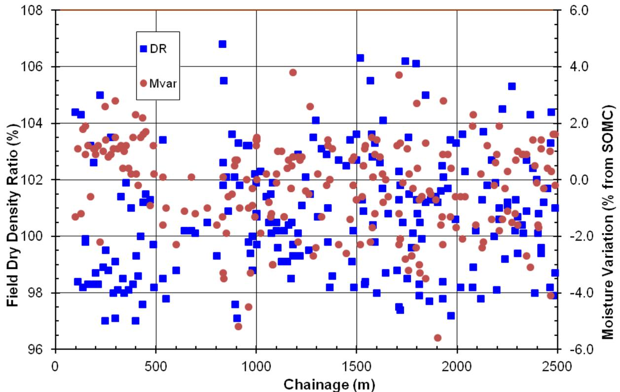
Figure 4. Spatial distribution of density-moisture test results for Western Levee
