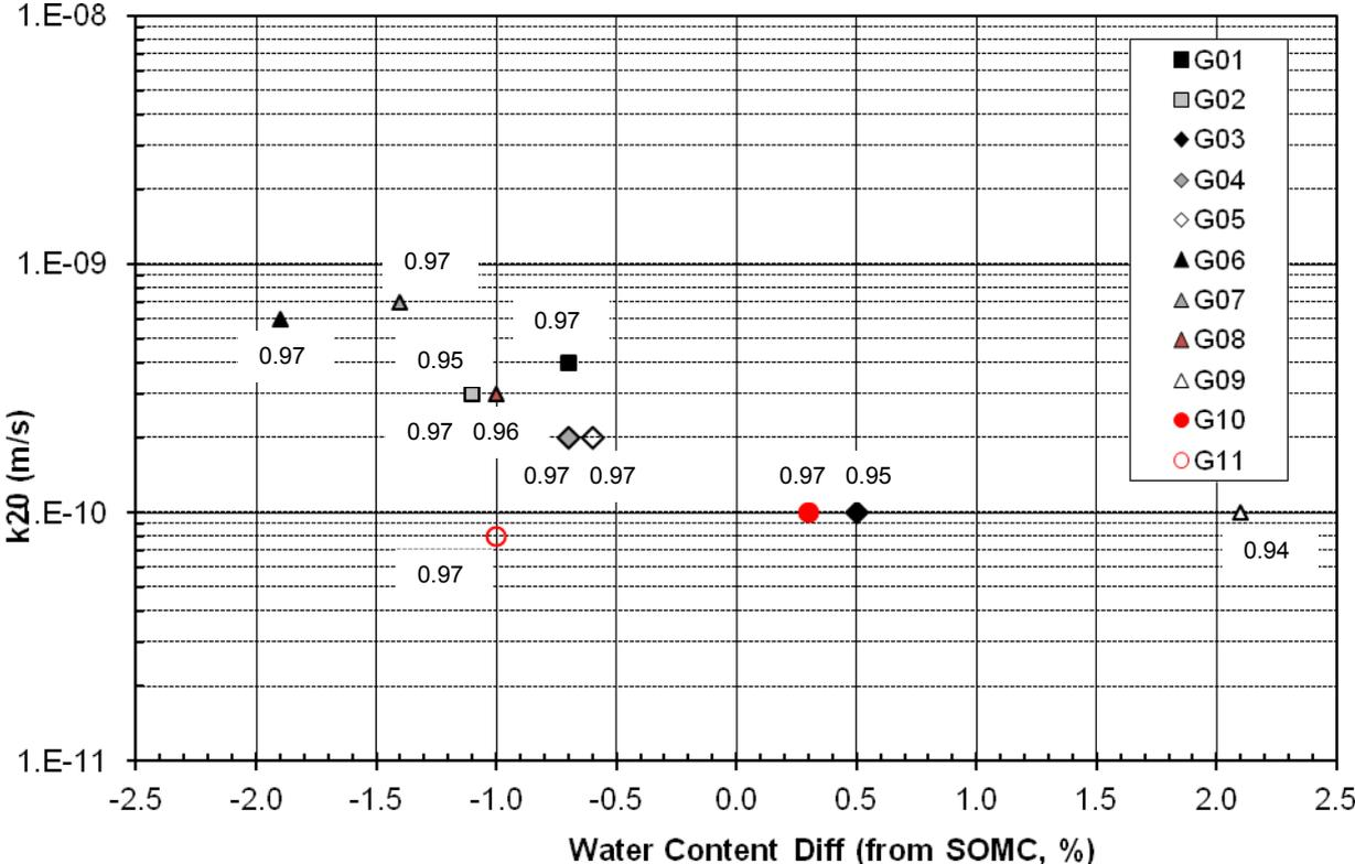
Figure 2. Laboratory saturated permeability results as functions of moisture and dry density condition
