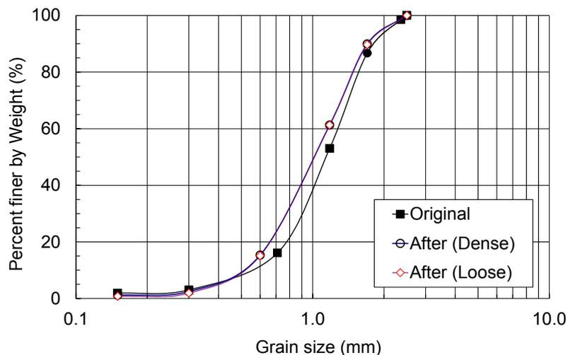
Figure 5. Grain size distribution curves before and after the cyclic tests.
