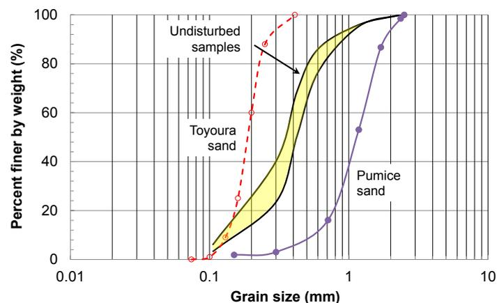
Figure 1. Grain size distribution curves of sands used in the tests.
