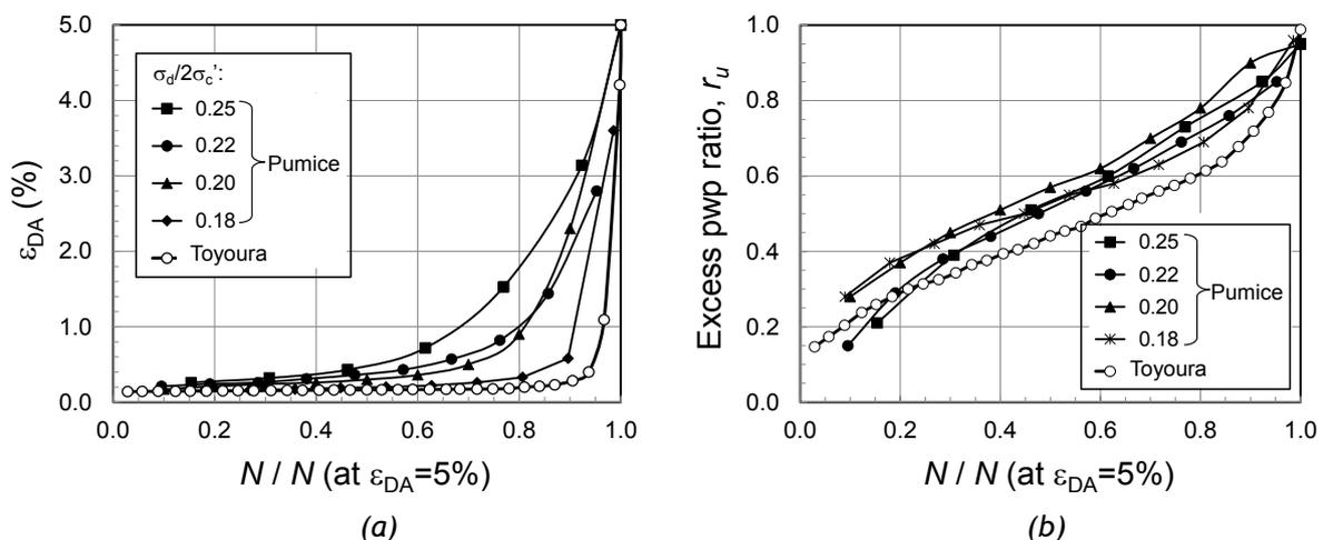
Figure 2. (a) Double amplitude axial strain  $\varepsilon_{DA}$  and (b) excess pore water pressure ratio  $r_u = u/\sigma_c'$  plots against normalized number of cycles  $N/N(\text{at } \varepsilon_{DA}=5\%)$  for loose pumice specimens.
