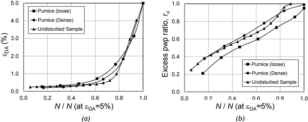
Figure 3. (a) Double amplitude axial strain  $\varepsilon_{DA}$  and (b) excess pore water pressure ratio  $r_u=u/\sigma'_c$  plots against normalized number of cycles  $N/N$ (at  $\varepsilon_{DA}=5\%$ ) for loose and dense reconstituted pumice sands and undisturbed specimens for  $\sigma_d/2\sigma'_c=0.25$ .
