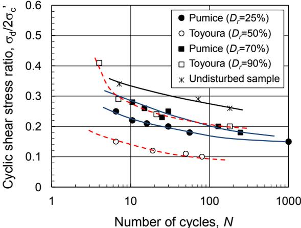
Figure 4. Cyclic resistance curves for the samples used.
