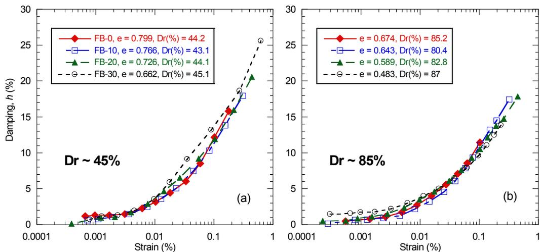
Figure 4. Damping curves for loose and dense sands with varying fines content
