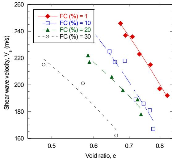
Figure 1. Linear best fit to shear wave velocity vs void ratio
