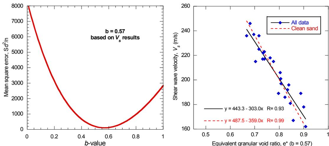
Figure 2. a) Determination of the best fit  $b$ -value based on shear wave velocity results, b) Shear wave velocity vs equivalent granular void ratio with  $b = 0.57$
