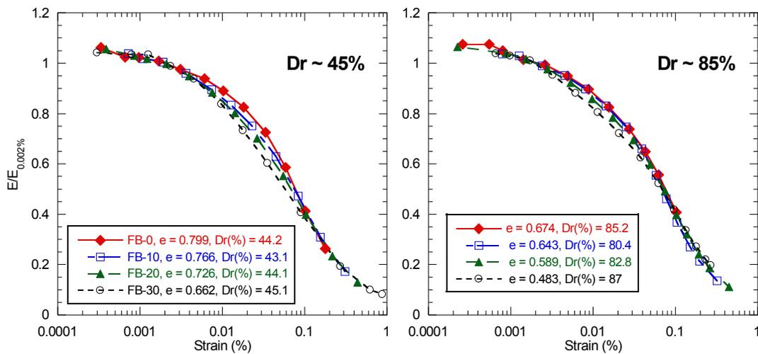
Figure 3. Normalized curves for loose and dense sands with varying fines content
