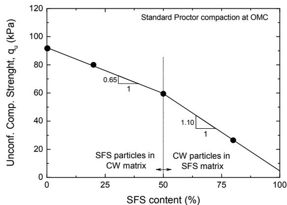
Figure 3. Variation of strength with SFS content for mixtures compacted at their OMC
