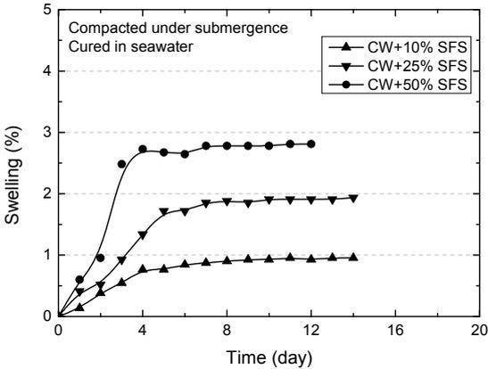
Figure 5. Swelling behaviour of various CW-SFS mixtures cured in seawater
