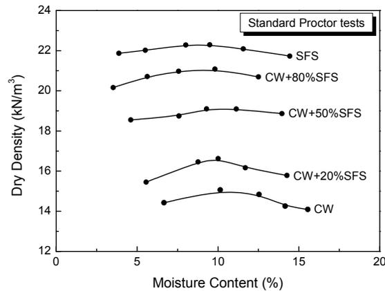
Figure 2. Compaction curves obtained for various CW-SFS mixtures
