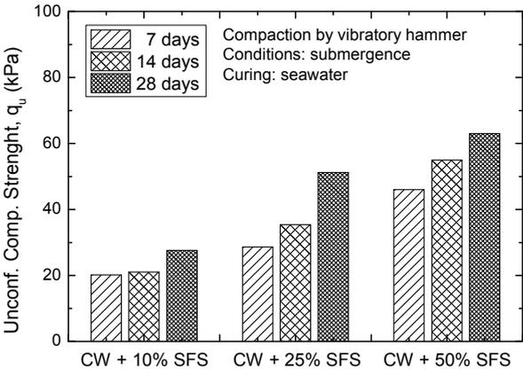
Figure 4. Variation of strength with curing time for various CW-SFS mixtures
